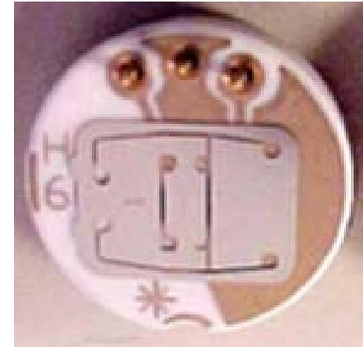
**the proof mass is suspended over the substrate by the two cantilever beams**
