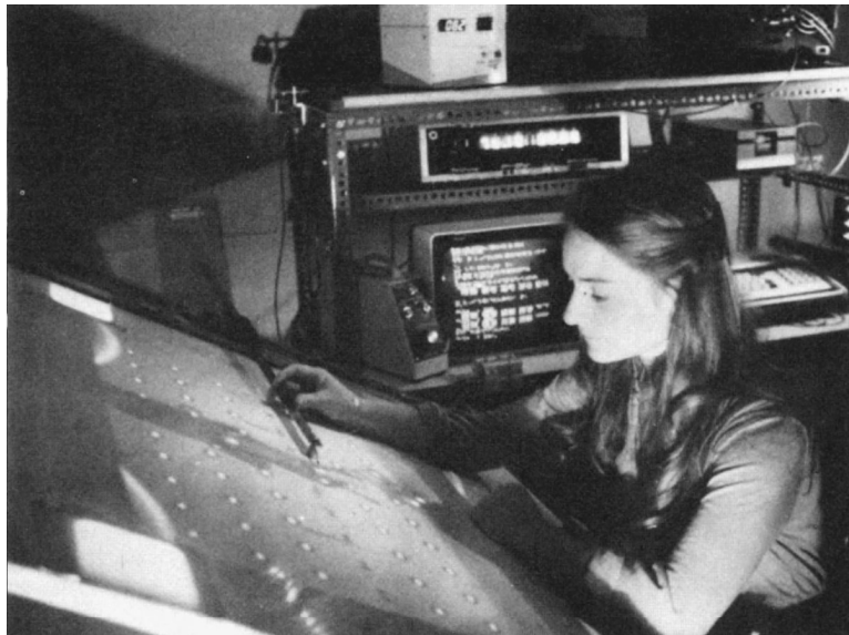
Figure 3.11 Typical arrangement for the microcomputer digitization of data coordinates from movie film. Foot pedal allows operator to transfer coordinate data to the computer at a rate of about 10 coordinate pairs per minute. Digitizing error is about 1 mm rms with the camera located 4 m from the subject.
