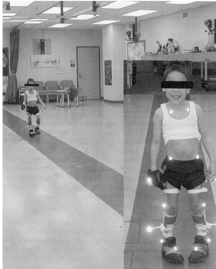
Figure 3.13 Gait assessment of a cerebral palsy patient in a clinical gait laboratory. Infrared cameras on the ceiling and walls capture the reflected light from the spherical reflective markers mounted on both sides of the body. (Courtesy of the Gait Analysis Laboratory, Connecticut Children's Medical Center, Hartford, CT.)
