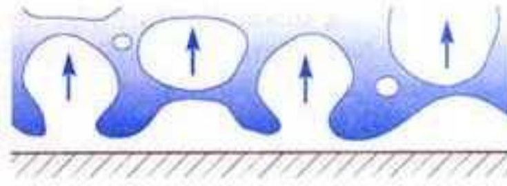
5. Stable film boiling
