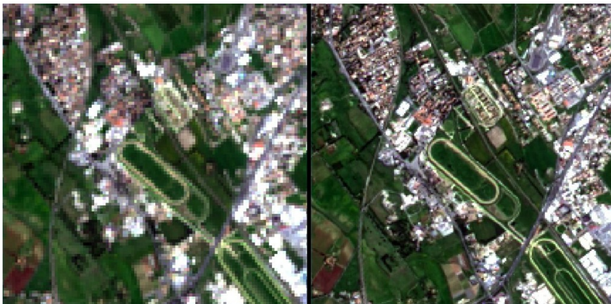
Fig. 12: Example of pan-sharpening of a Landsat 8 image. Left, original multispectral bands (30m); right, pan-sharpened bands (15m)
