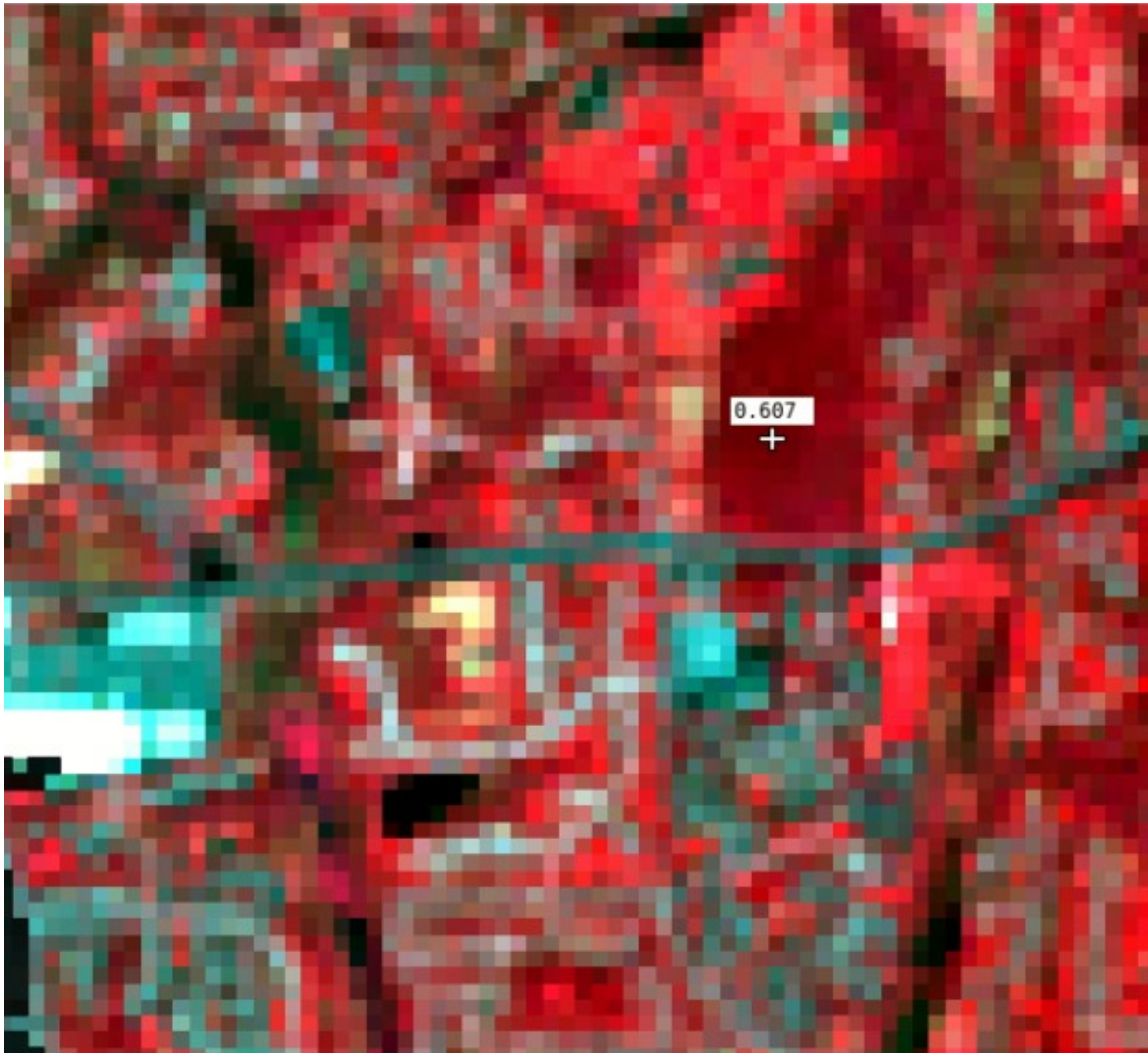
Fig. 19: NDVI value of vegetation pixel displayed in the map. Color composite RGB = 4-3-2
