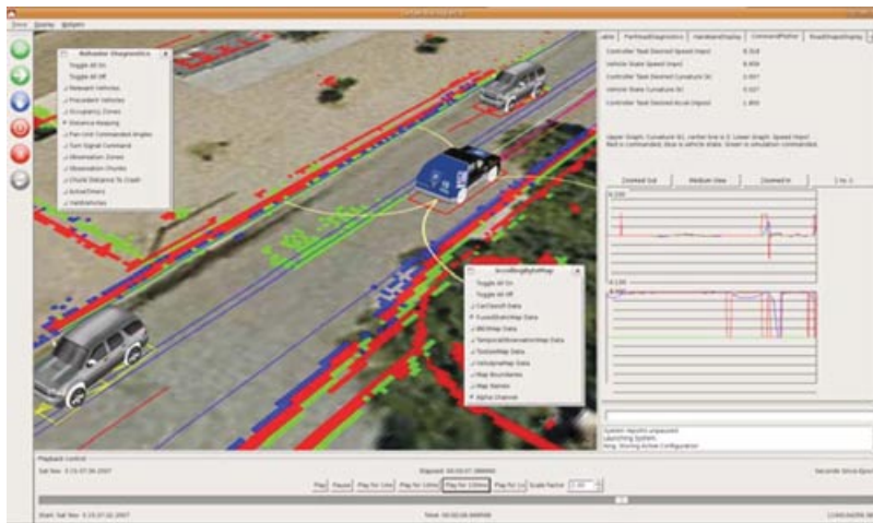
Figure 23. The TROCS is an extensible GUI that enables developers to both monitor telemetry from Boss while it is driving and replay data offline for algorithm analysis.
