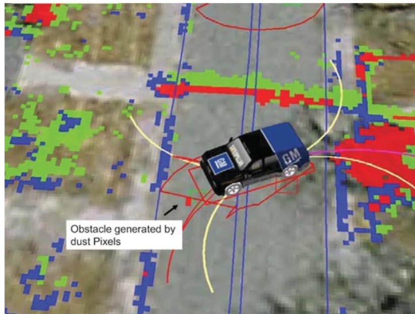
Figure 29. The false obstacles generated by dust and the bush behind Boss prevented Boss from initially completing its U-turn.
