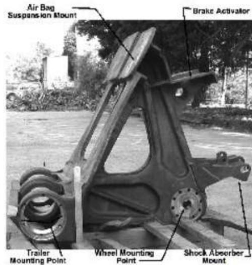
A truck trailer suspension arm made from austempered ductile iron, Steele and Lincoln Foundry.
