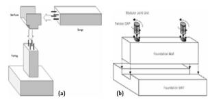
Fig.3. Foundation System - (a) Independent foundation. (b) Wall foundation.
