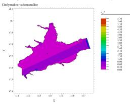
Fig.4. Concentration of phosphate in Rostov part of Tsimlyansk Reservoir
