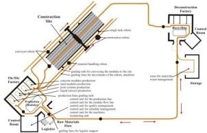
Figure 30: Automated Construction (On-site factory and construction). (own concept).
