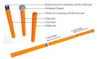
Figure 15: Proposed design for the piles.
