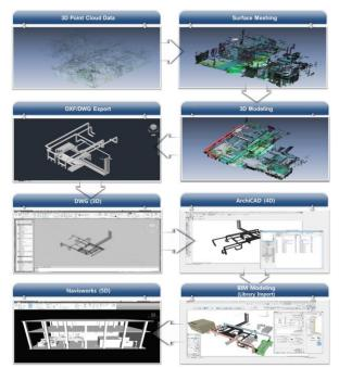
Fig.1. In-situ as-building model acquisition process
