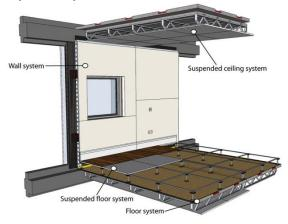
Fig.3. UCS wall, floor components design
