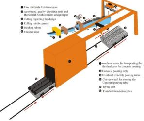
Figure 16: Production line construction process for foundation piles (own concept).
