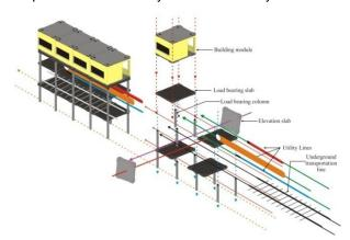
*Figure 32: modularization and construction process. (own concept).*
