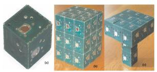
Fig.2. Miche system: (a)Single module (b)Initial uniform assembly of modules (c)Obtained desired assembly.
