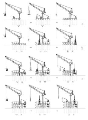
Fig.6. UCS construction evolution scheme
