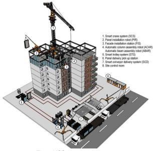
Fig.5. UCS construction system
