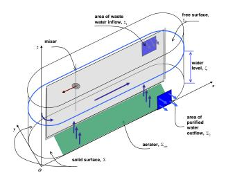
Fig.7. The scheme of circular bio-aeration tank
