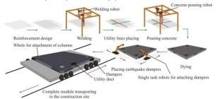
Figure 17: Production line construction process for load bearing slabs (own concept).
