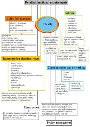
Figure 11: Detailed Functional Requirements for a city.
