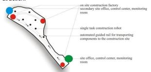
Figure 34: Schematic drawing for Automated on site factory, supply line, control center and automated logistic
