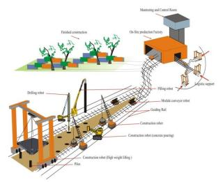
Figure 27: Automated Construction (On-site factory and construction). (own concept).
