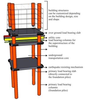
Figure 13: Figure shows the whole module. This should be the one module. Joining more modules together will create the whole city.
