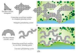
Figure 22: Several Modular approaches for the planning flexibility for a city design; (A) cube/ rectangular planning system, (B) honeycomb/ hexagonal planning system, (C) triangular planning system, (D) planning with curvature system and (E) using different systems at a time achieving flexibility of planning (own concept)..
