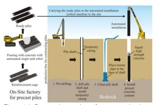
Figure 14: Proposed procedures for constructing large diameter bored piles (automated way).
