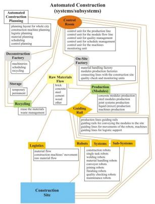
Figure 26: Automated Construction (systems and subsystems) (own concept).
