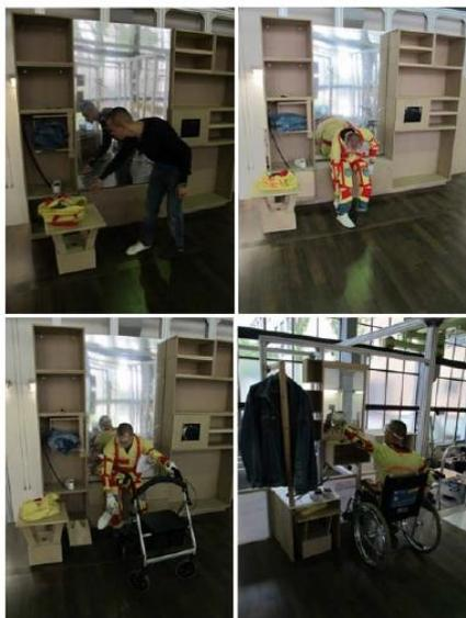
Fig. 1. Evaluation of the robotic furniture system by an age simulation suite<sup>2</sup>
