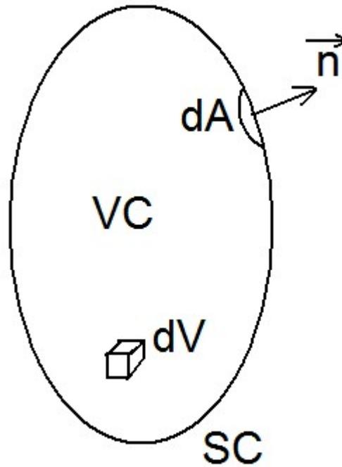
$$\int_{V(t)} \rho \frac{D\phi}{Dt} dV = \int_{VC} \frac{\partial(\rho\phi)}{\partial t} dV + \int_{VC} \nabla \cdot (\rho \vec{u} \phi) dV \quad (1.6)$$
