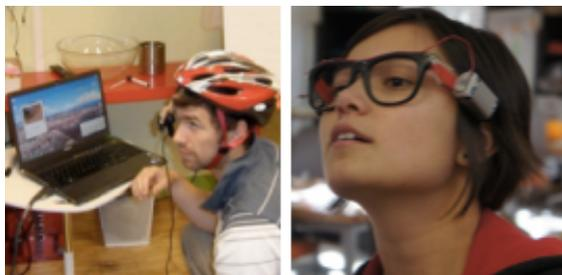
Figure 1 ParisTech and Stanford students test a helmet and glasses that shift the focus and perspective of an image based on the user's movement, elements of the team's initial product vision.
