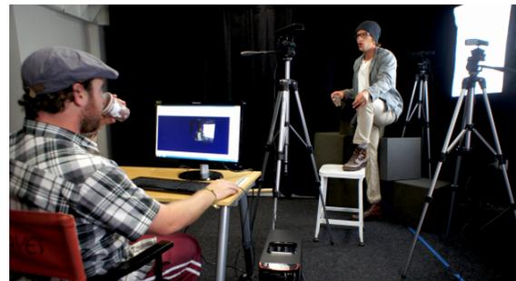
Figure 2 A director tests a refined version of the Thales team's Dark Horse scene-capturing setup, including multiple Microsoft Kinects and a compilation of software.
