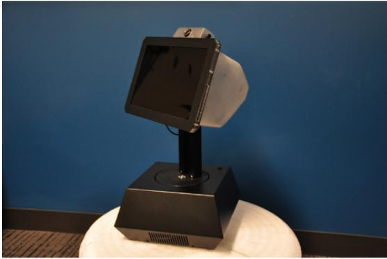
Figure 5 The Swisscom team's final functional prototype, a videoconferencing unit that allows participants to control the viewing angle remotely. This critical design element evolved directly from their Dark Horse prototype.
