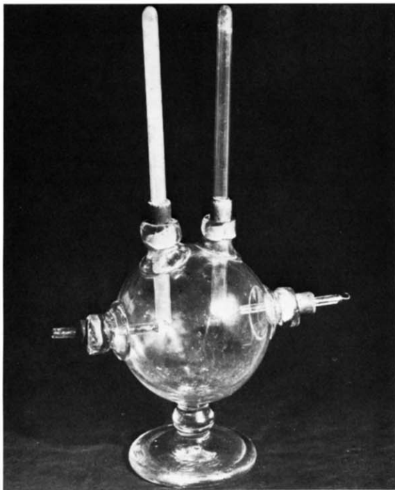
Figure 1. Voltammeter (coulometer) used by Faraday (by permission of the Director, Royal Institution of Great Britain).
