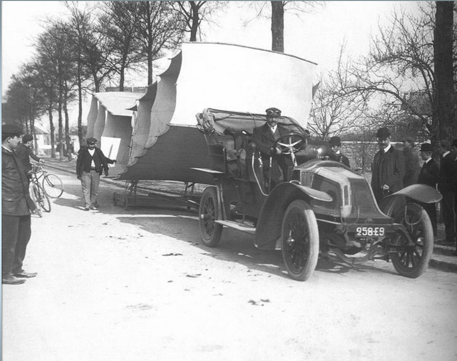
The 14-Bis wing being transported by a car (Reproduced from Musa, Mourão and Tilkian, 2003).
