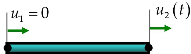
$$\frac{\rho AL}{6} \begin{bmatrix} 2 & 1 \\ 1 & 2 \end{bmatrix} \begin{Bmatrix} \ddot{u}_1 \\ \ddot{u}_2 \end{Bmatrix} + \frac{AE}{L} \begin{bmatrix} 1 & -1 \\ -1 & 1 \end{bmatrix} \begin{Bmatrix} u_1 \\ u_2 \end{Bmatrix} = \begin{Bmatrix} 0 \\ 0 \end{Bmatrix}$$
