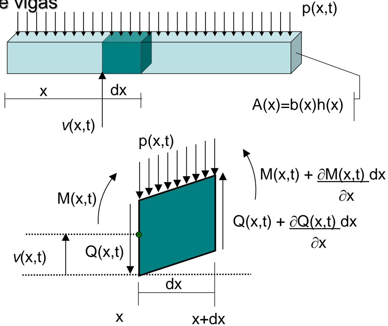
$$\frac{\partial Q}{\partial x} = p(x,t) - m\ddot{v}(x,t) - c\dot{v}(x,t) \quad \frac{\partial M}{\partial x} = Q \quad M = EIv''$$
