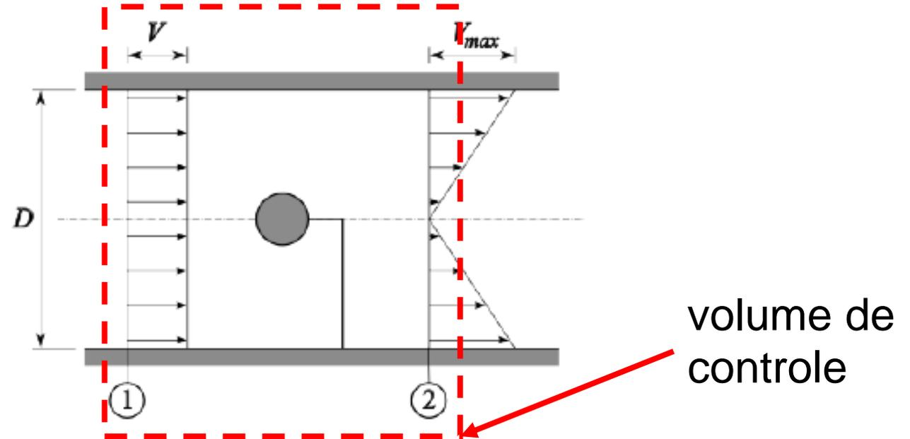
$$\rho_{\text{água}} g (p_1 - p_2) \frac{\pi D^2}{4} + F_{\text{arrasto}} = \rho_{\text{ar}} v \frac{\pi D^2}{4} (-v) + \underbrace{\int_0^{D/2} \rho_{\text{ar}} 2\pi R (30R)^2 dR}_I$$
