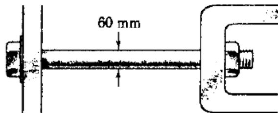
2.66 The change in diameter of a large steel bolt is carefully measured as the nut is tightened. Knowing that  $E = 200$  GPa and  $\nu = 0.29$ , determine the internal force in the bolt, if the diameter is observed to decrease by  $13 \mu\text{m}$ .
