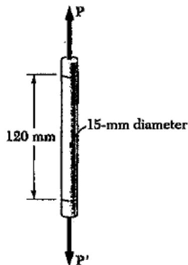
2.64 A standard tension test is used to determine the properties of an experimental plastic. The test specimen is a 15-mm-diameter rod and it is subjected to a 3.5 kN tensile force. Knowing that an elongation of 11 mm and a decrease in diameter of 0.62 mm are observed in a 120-mm gage length, determine the modulus of elasticity, the modulus of rigidity, and Poisson's ratio of the material.
