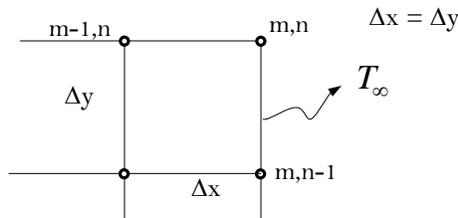
$$2T_{m,n} \left( h \frac{\Delta x}{k} + 1 \right) - 2h \frac{\Delta x}{k} T_{\infty} - (T_{m-1,n} + T_{m,n-1}) = 0$$
