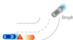
Blind curve/ Local hazard warning
