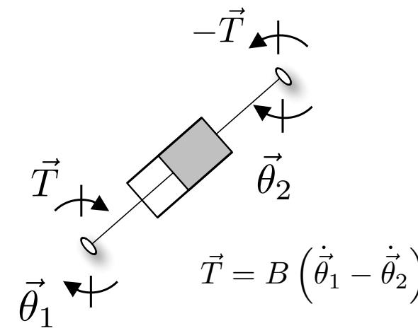
$$\begin{array}{c} \vec{f} \quad \vec{T} \\ \vec{u} \quad \vec{\theta} \end{array} \rightarrow \boxed{\begin{matrix} \frac{1}{Bs} & \frac{1}{Bs} \\ Bs & Bs \end{matrix}} \rightarrow \begin{array}{c} \vec{u} \\ \vec{f} \end{array} \rightarrow \begin{array}{c} \vec{\theta} \\ \vec{T} \end{array}$$
