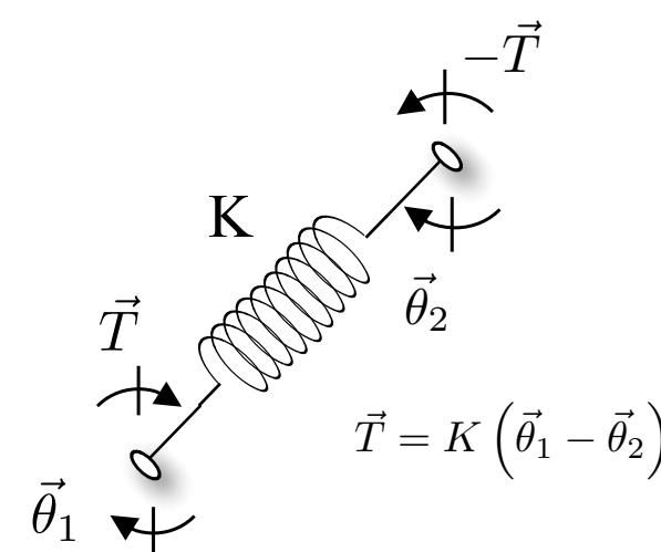
$$\begin{array}{c} \vec{f} \quad \vec{T} \\ \vec{u} \quad \vec{\theta} \end{array} \rightarrow \boxed{\begin{matrix} \frac{1}{K} & \frac{1}{K} \\ K & K \end{matrix}} \rightarrow \begin{array}{c} \vec{u} \\ \vec{f} \end{array} \rightarrow \begin{array}{c} \vec{\theta} \\ \vec{T} \end{array}$$
