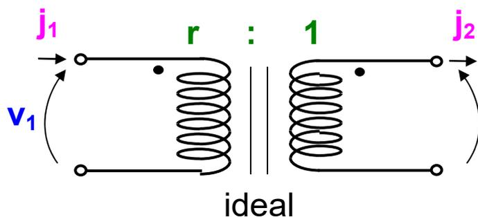
$$\frac{v_2}{v_1} = \frac{1}{r}$$
