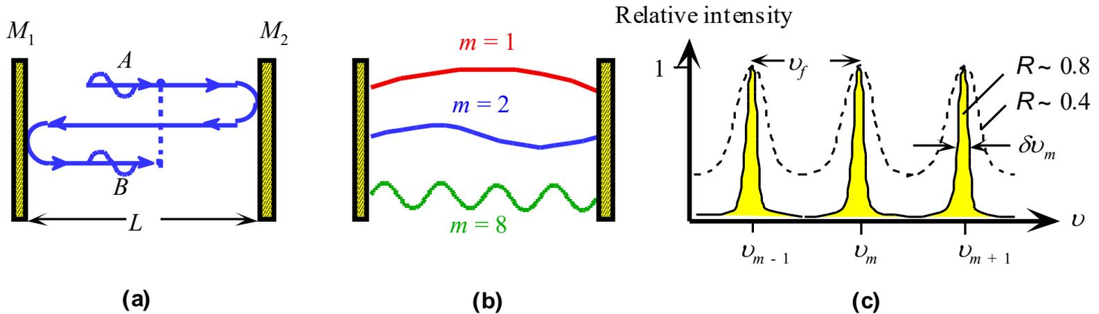
Schematic illustration of the Fabry-Perot optical cavity and its properties. (a) Reflected waves interfere. (b) Only standing EM waves, *modes*, of certain wavelengths are allowed in the cavity. (c) Intensity vs. frequency for various modes.  $R$  is mirror reflectance and lower  $R$  means higher loss from the cavity.
