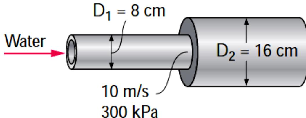
**Solution** A horizontal water pipe has an abrupt expansion. The water velocity and pressure in the smaller diameter pipe are given. The pressure after the expansion and the error that would have occurred if the Bernoulli Equation had been used are to be determined.
