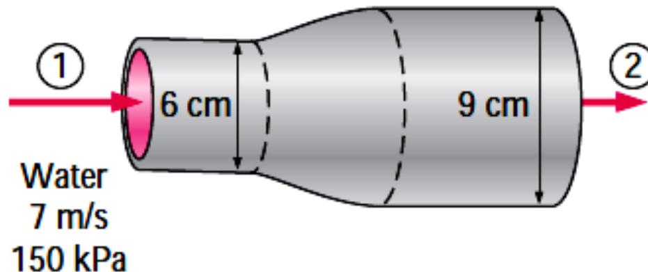
**SOLUTION** A horizontal water pipe expands gradually into a larger-diameter pipe. The head loss and pressure after the expansion are to be determined.
