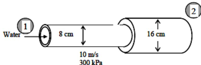
Therefore, despite the head (and pressure) loss, the pressure increases from 300 kPa to 321 kPa after the expansion. This is due to the conversion of dynamic pressure to static pressure when the velocity is decreased.
