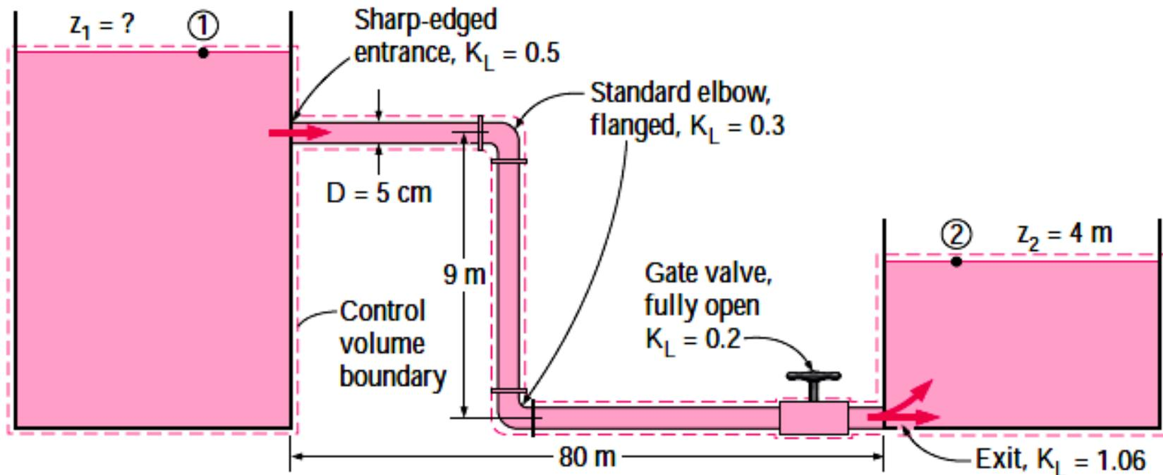
**SOLUTION** The flow rate through a piping system connecting two reservoirs is given. The elevation of the source is to be determined.
