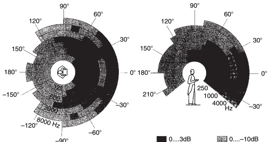
Fig. 4.33 Angular regions of principal radiation regions of the singing voice in octave bands (after Marshall and Meyer, 1985)
