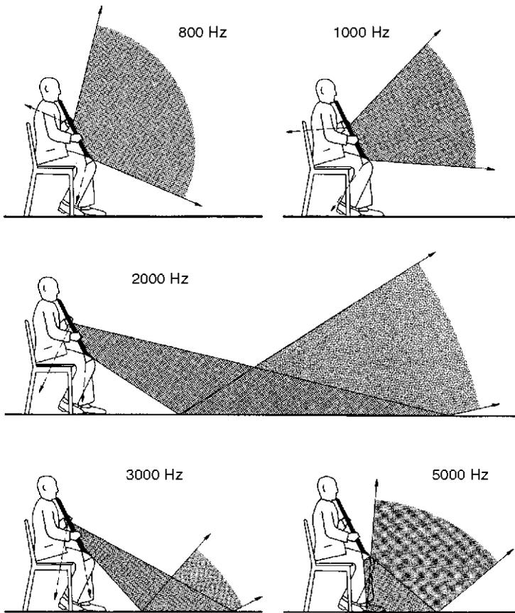
Fig. 7.20 Principal radiation directions (0...-3 dB) for clarinets
