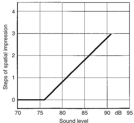
**Fig. 5.14** Limiting value of sound levels for onset of spatial impression. Data points for onset of spatial impression. Data points for onset of spatial impression. Data points for onset of spatial impression (After Kuhl, 1978) from top to bottom: Stadthalle Hannover, Rheinhalle Düsseldorf, Philharmonie Berlin, Musikhalle Hamburg, Stadthalle Wuppertal. The lowest data point refers to hearing tests with electroacoustic instrumentation
