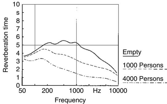
**Fig. 6.25** Reverberation curve of the Frauenkirche in Dresden (after Lottermoser, 1960). *Empty*: measured from historic tape-recordings. *Occupied*: calculated from the curve for the empty church (Mozarteum Salzburg)
