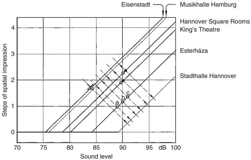
**Fig. 8.4** Spaciousness of the orchestral sound in six concert halls in dependence on sound level. The average *forte* level of historical orchestras is given by circles (without clarinets) or dots (with clarinets). a Esterháza 1766–1774, b 1775–1780, c after 1780. Broken lines: lines of equivalent *forte* impressions
