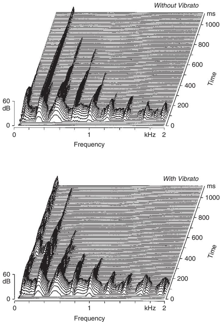
**Fig. 3.20** Influence of *vibrato* on time evolution of the tonal spectrum of a string *pizzicato* (Violin, B<sub>3</sub>)
