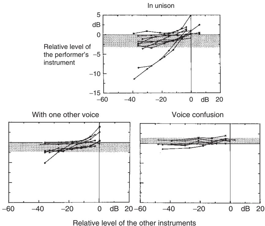
**Fig. 8.8** Influence of mutual listening on the radiated sound level: performance strength of individual violinists for varying loudness of other voices. Reference value (0 dB for both axes) is the sound level of the instrument when no other voices are present (after Naylor, 1987)
