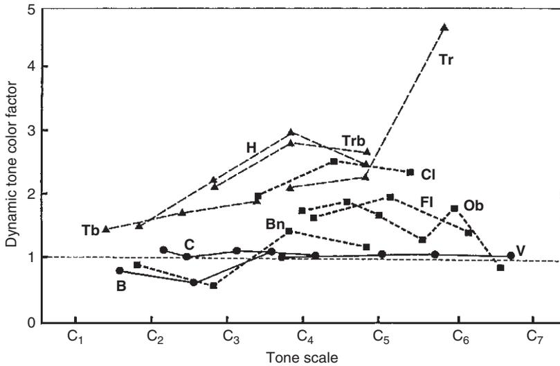
Fig. 8.6 Dynamic tone color factor (relationship of level change of 3,000 Hz components to the level change of its strongest partials) for orchestral instruments in dependence on pitch
