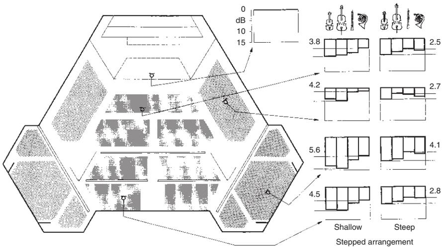
**Fig. 7.42** Level differences between different audience locations and the location of the conductor for four instrument sections and two types of orchestral seating (Stadthalle Braunschweig)
