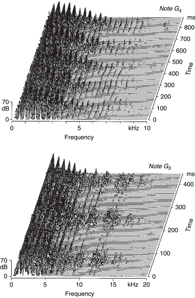
Fig. 3.9 Time variations in the tonal spectrum of a flute vibrato for different pitch regions
