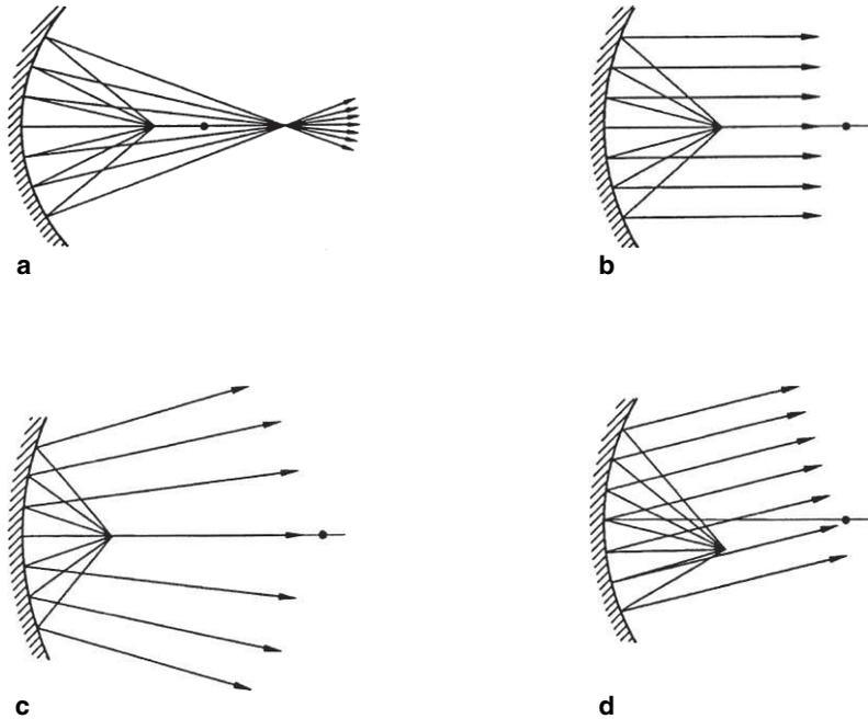
Fig. 5.2 Reflection from curved surfaces
