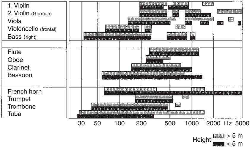
**Fig. 6.10** Frequency regions of preferred rear wall reflections for orchestra instruments
