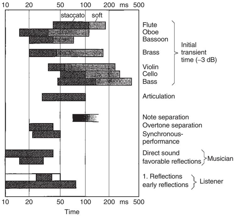
Fig. 8.11 Characteristic regions for time structure of tone onsets
