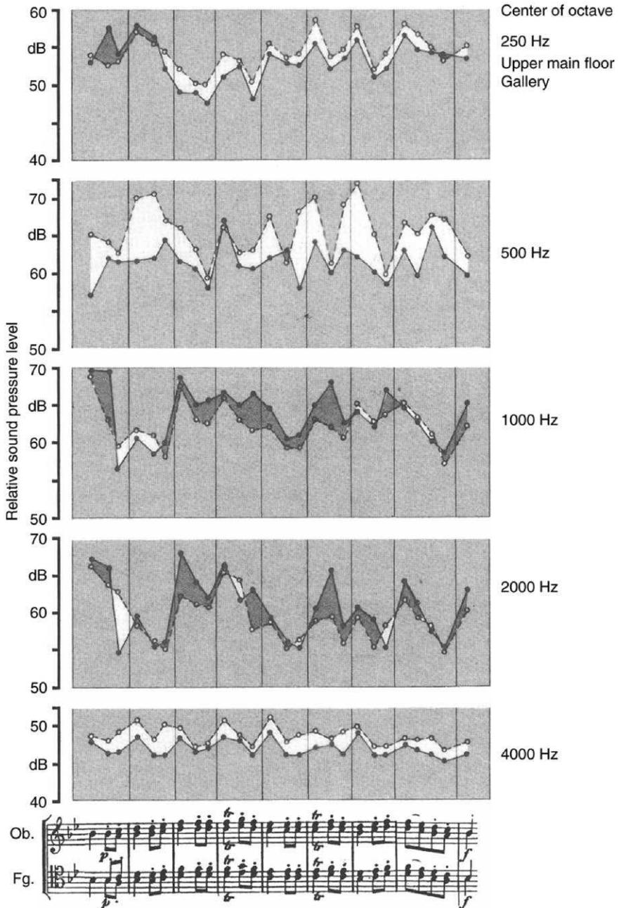
**Fig. 7.23** Octave level analysis of a passage for two oboes and two bassoons (W.A. Mozart, Symphony B<sup>b</sup> major, K319, 4th Movement, measure 336–344) in two locations in the large hall of the Stadthalle Braunschweig
