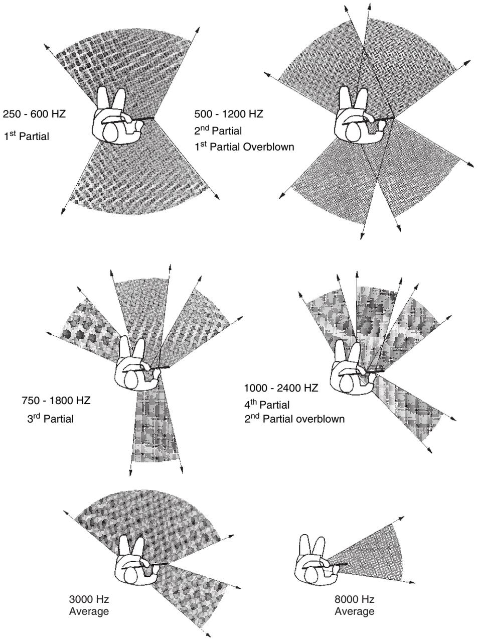
Fig. 7.17 Principal radiation directions (0...-3 dB) of flutes
