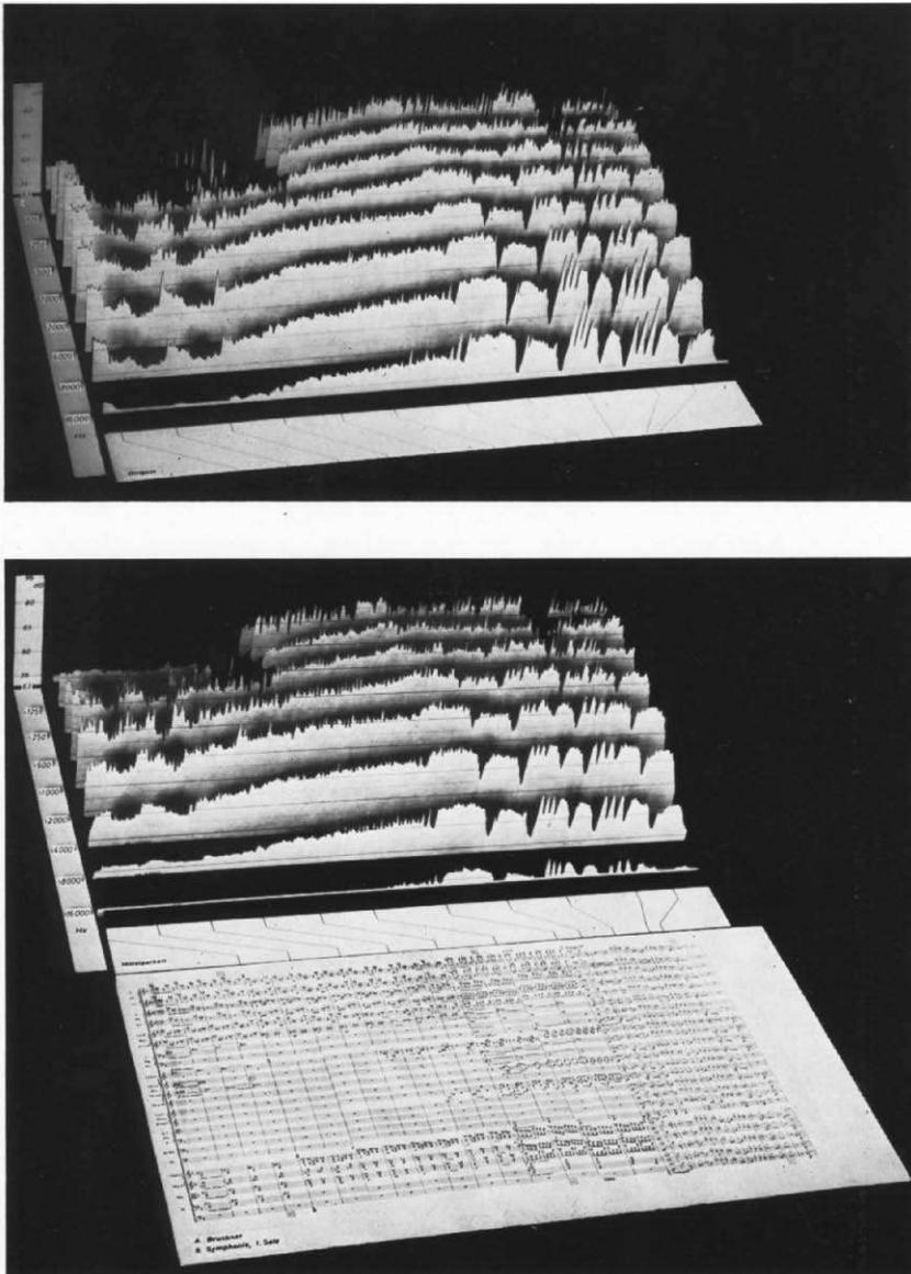
**Fig. 7.31** Octave level models of the orchestral sound in the Stadthalle Braunschweig (A. Buckner, 9th symphony, 1st movement, measure 51–71). *Top*: sound at conductor location. *Bottom*: sound in the 5th row of the main floor
