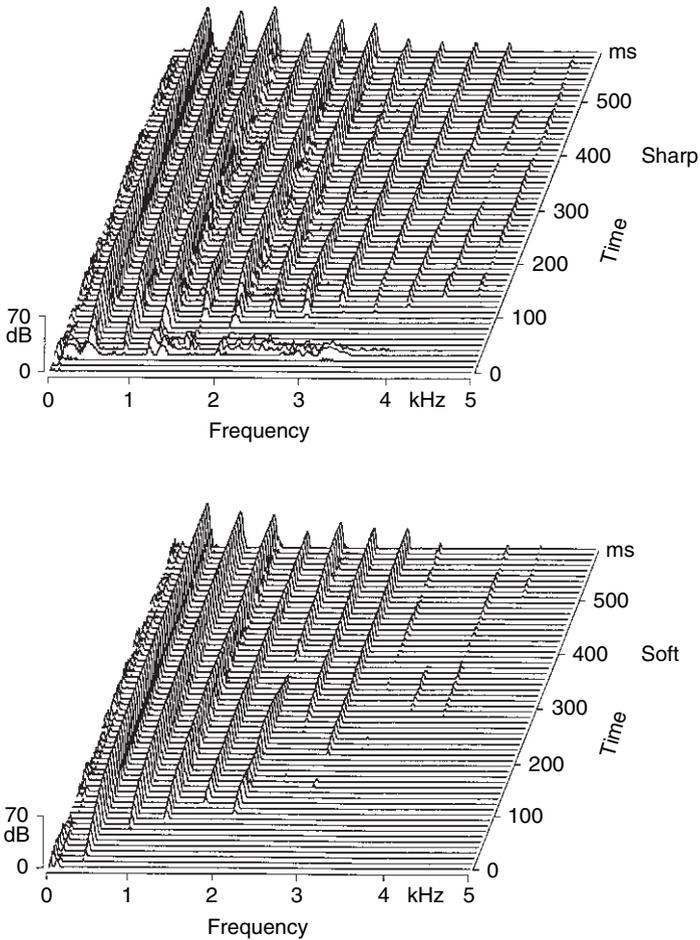
Fig. 2.9 Time development of a tone spectrum for different attacks (Flute, G<sub>4</sub>)
