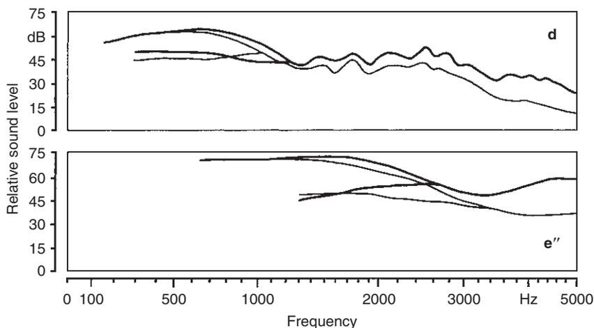
**Fig. 8.17** Envelopes of sound spectra of a clarinet for different instrument positions recorded in direction of sight (*horizontal*) of the player. *Thin line*: normal position; *thick line*: bell raised
