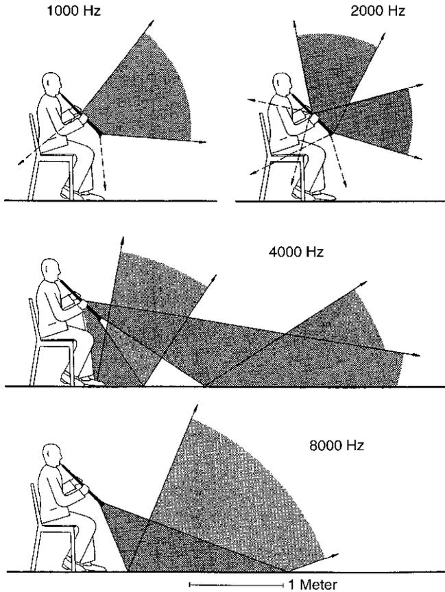
Fig. 7.19 Principal radiation directions (0...-3 dB) for oboes
