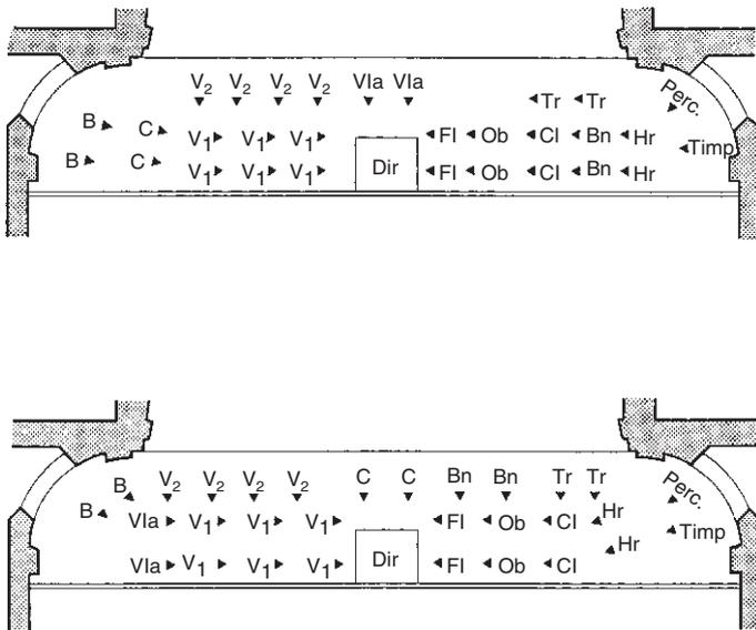
Fig. 9.5 Seating arrangement of the opera orchestra in the “Schloßtheater Drottningholm” for a Mozart opera. Top: customary seating in 1969. Bottom: seating arrangement improved, based on acoustic principles
