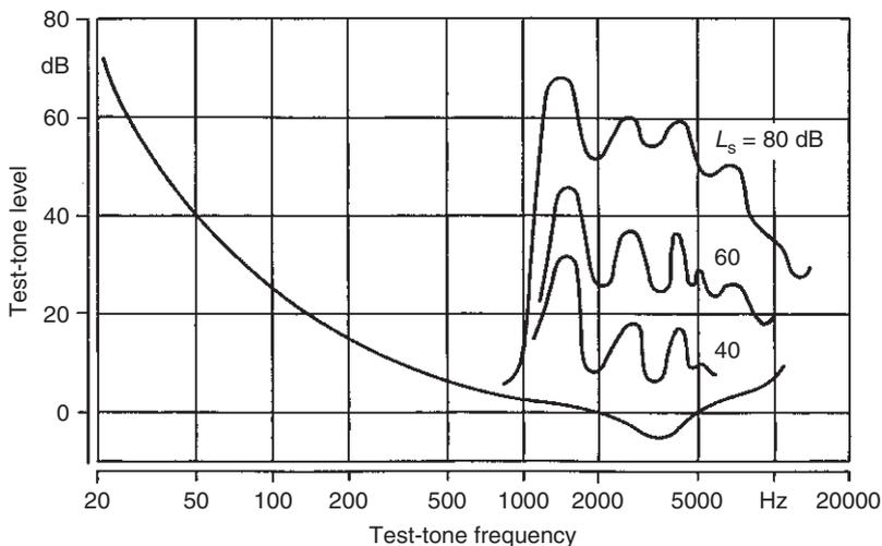
**Fig. 8.10** Masked threshold of a sinusoidal tone (“test tone”) which is masked by high violin tones performed with variable loudness (After Zwicker, 1982)
