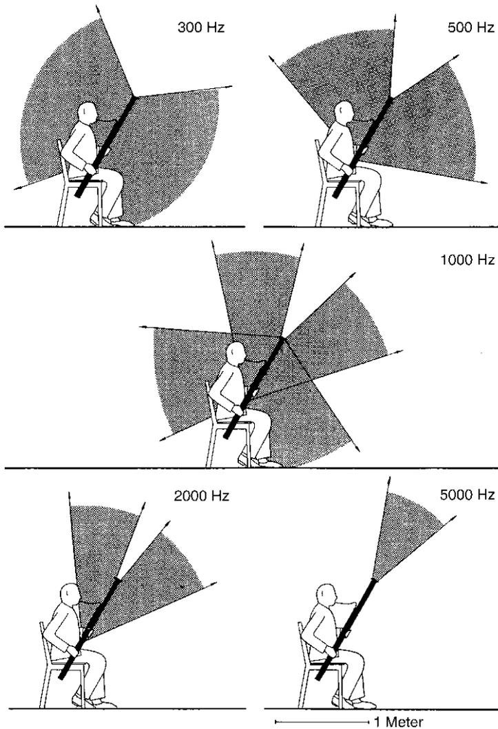
Fig. 7.22 Principal radiation directions (0...-3 dB) for bassoons
