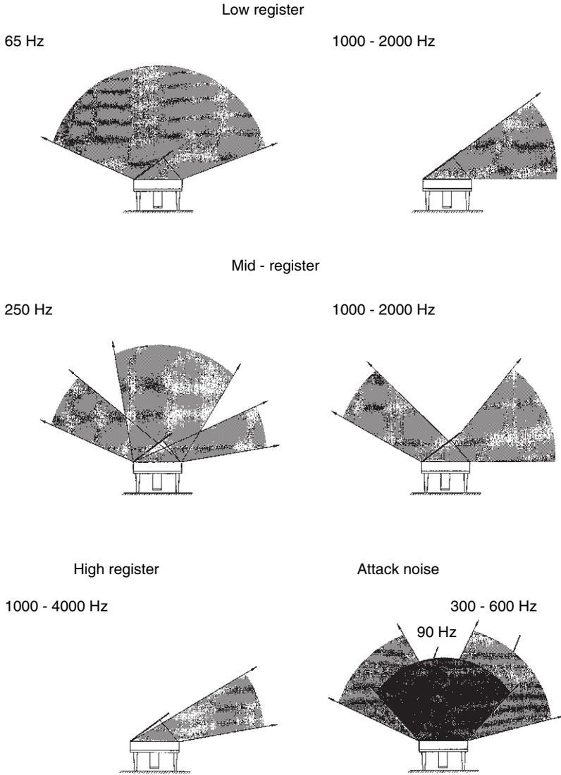
**Fig. 7.38** Principal radiation directions (0...-3 dB) of a concert grand piano for the most important partials and the attack noise
