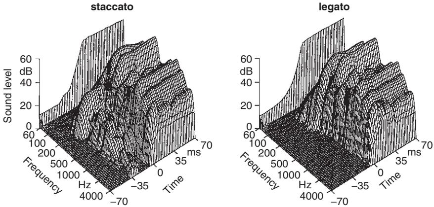
**Fig. 3.22** Influence of attack technique on the noise components of initial transients for a grand piano (played tone: C<sub>3</sub>; after Koornhof and van der Walt, 1993)
