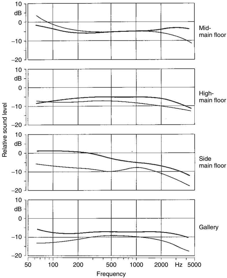
**Fig. 7.43** Level difference of celli in different hall locations in relationship to the level at the location of the conductor. (Stadthalle Braunschweig). *Thin line:* seating with shallow steps; *thick line:* seating with steep steps
