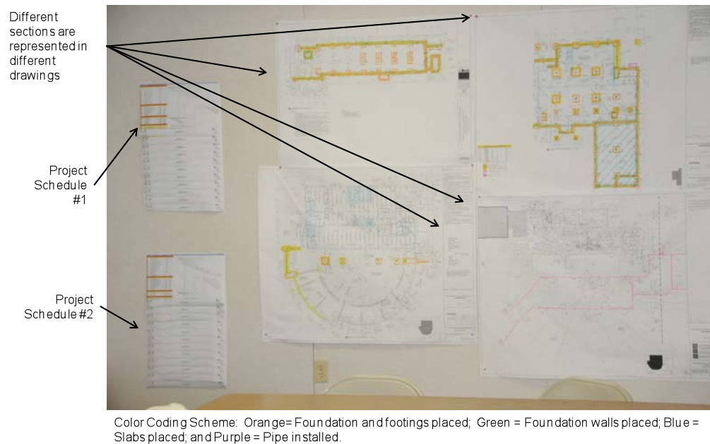
FIG. 2: An example of existing progress reporting techniques. Construction drawings and work schedules are hung on a construction site trailer's wall to communicate progress with contractors and subcontractors. Progress is visualized in two-dimensional drawings using annotations and color-coding. The date on which progress is made is also annotated on different sections. Different work plans are hung over each other.
