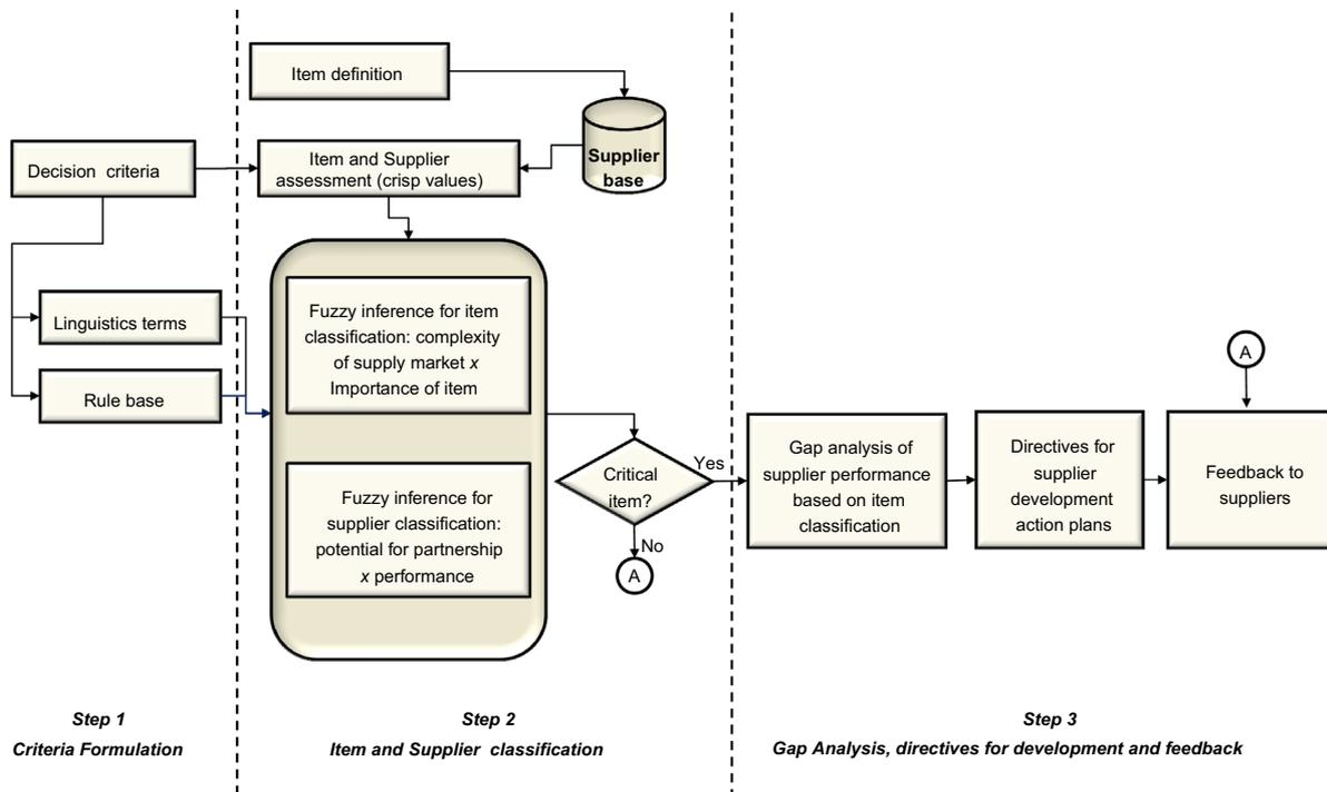
Fig. 4. Framework of the proposed method for supplier evaluation.
