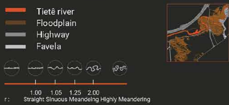
Sinuosity Coefficient (R) = Curvilinear Length [CL] / Euclidean Distance [ED] Channelization and rectification of the Tietê river over 113 years
