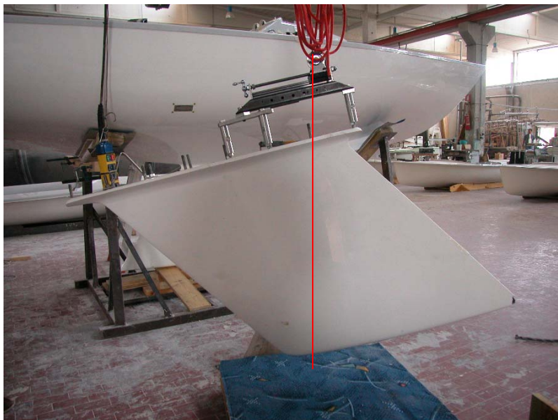
Figure 26. A keel suspended from a swing bearing for center of mass and pitch gyradius measurement.
