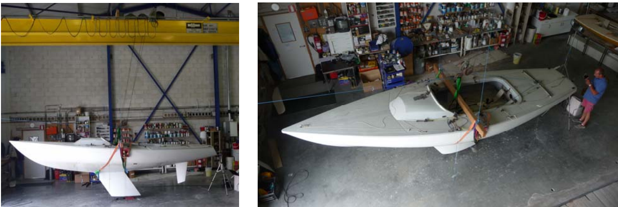
Figure 5. The hull suspended for the yaw test. The two cross beams with eyebolts to which the supporting lines are attached can be seen. The vertical photogate used for timing is mounted on the tripod at the stern (the rudder was reversed before measurement!).
