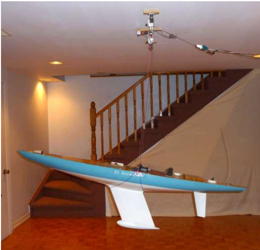
Figure 30 A model sailboat hull in pitch-surge-heave double pendulum oscillation.
