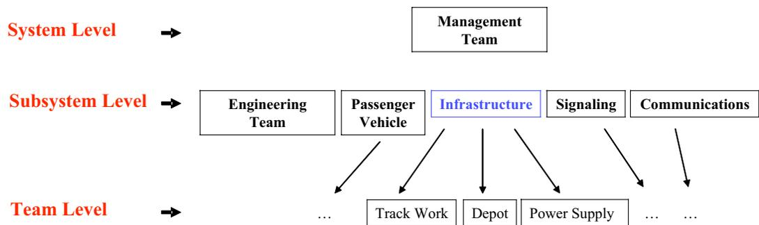
**Figure 4.4: System and subsystem level in the MRT Project**
