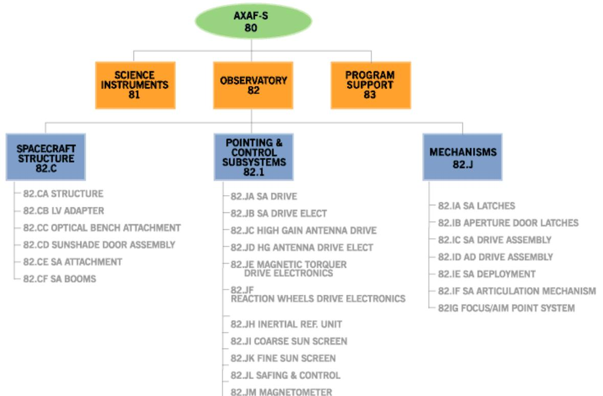
**Figure 2.6: Product-Oriented WBS for the NASA's AXAF Spectrometer Spacecraft**
