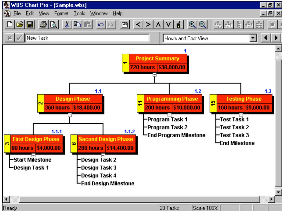
Figure 5.1: A sample WBS using the WBS Chart Pro Software
