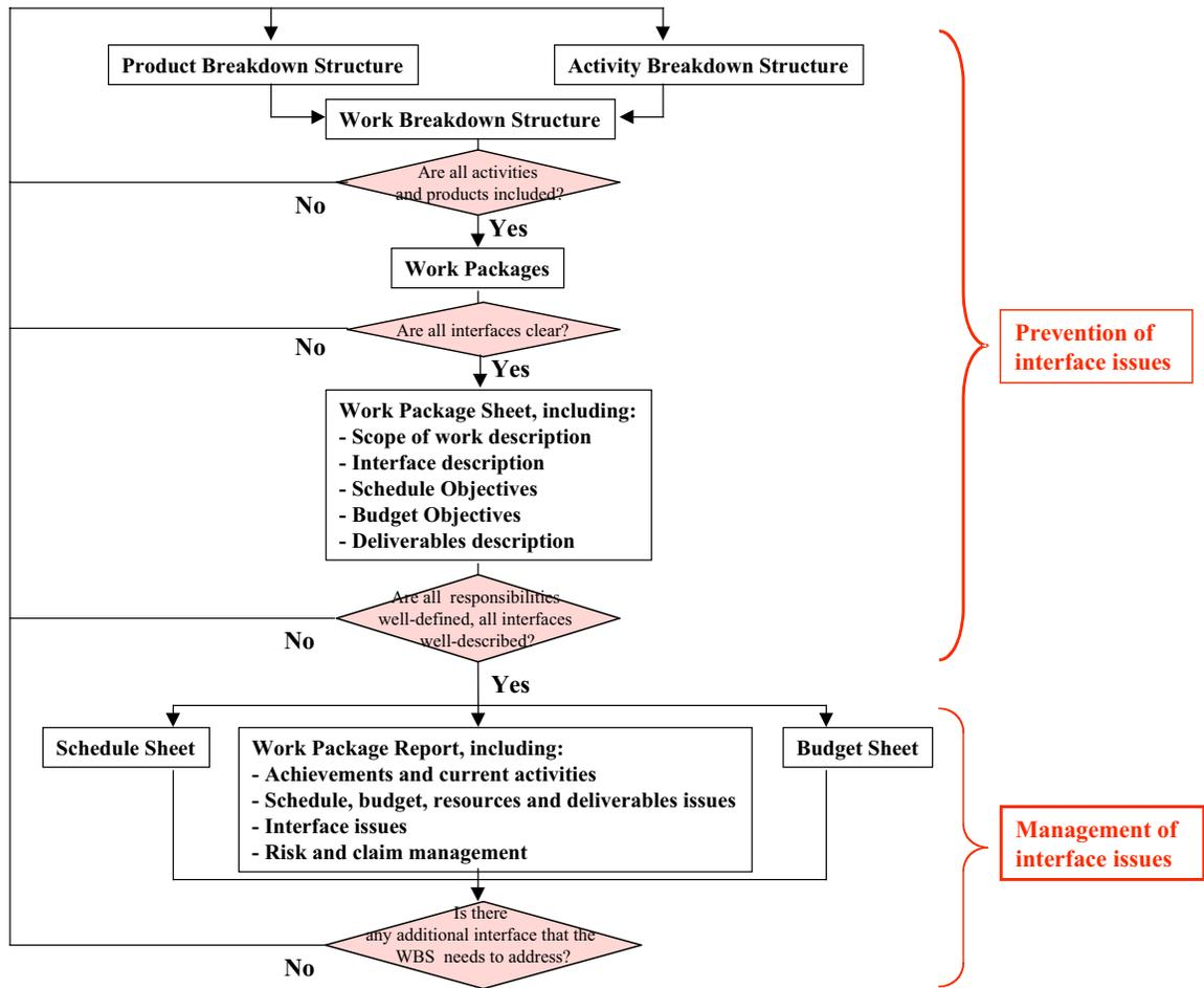
**Figure 3.2: Components of a WBS matrix management package**
