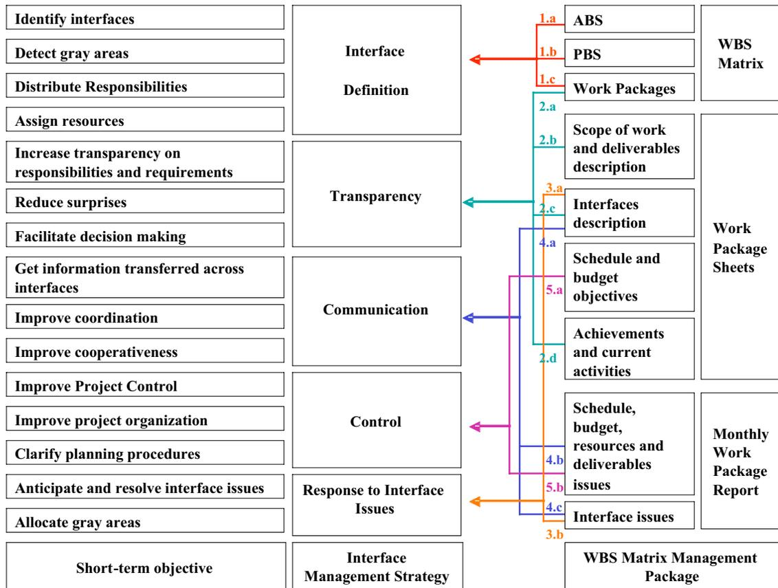
**Figure 4.15: Different possible uses of a WBS matrix management package for interface management**
