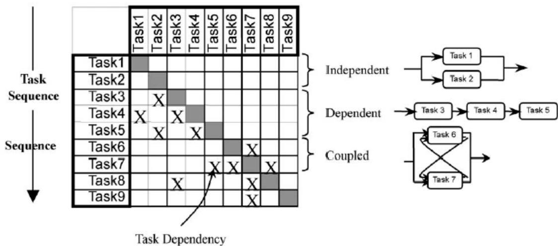
**Figure 2.3: Sample task-based DSM matrix, with explanations on the relationships between tasks (taken from Chun-Hsien et al., 2003)**
