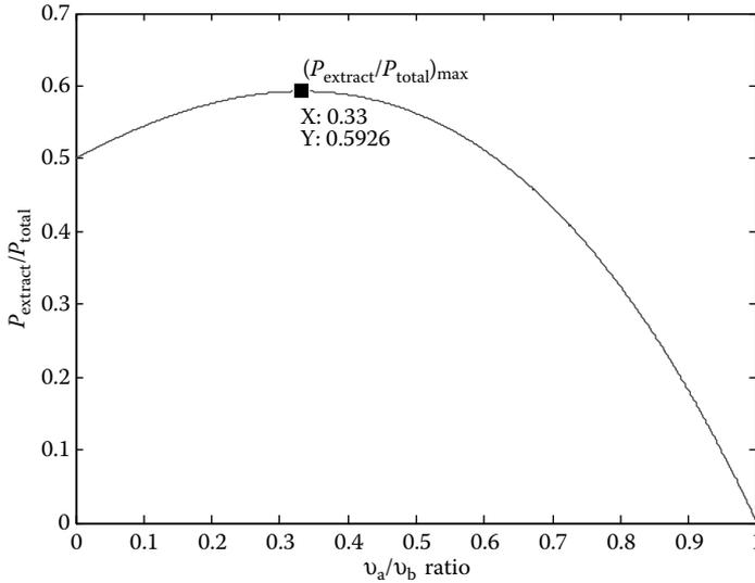
FIGURE 2.5 Maximum theoretical extracted power from wind.
