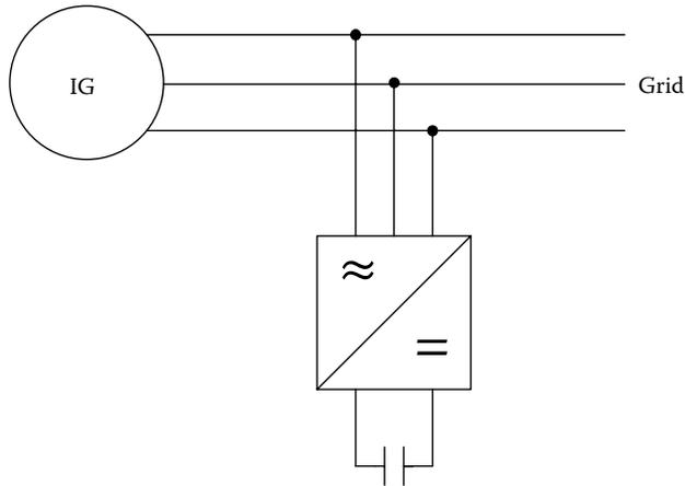
FIGURE 4.64 Induction generator with a shunt connected STATCOM.
