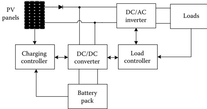
FIGURE 1.74 PV/battery connection—type 2.
