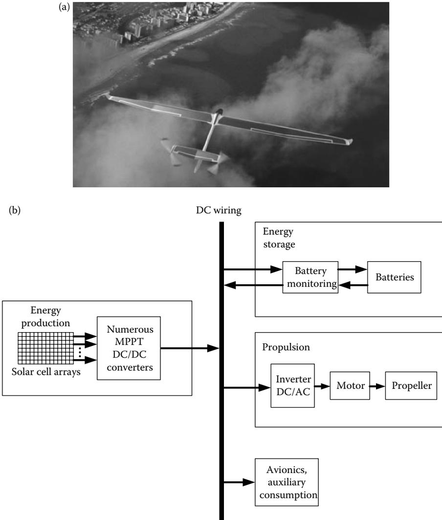
**FIGURE 1.110** (See color insert following page 80 for [a].) (a) Solar-powered aircraft and (b) aircraft power train. (Modified from Y. Perriard, P. Ragot, and M. Markovic, *IEEE International Conference on Electric Machines and Drives*, pp. 1459–1465, May 2005.)
