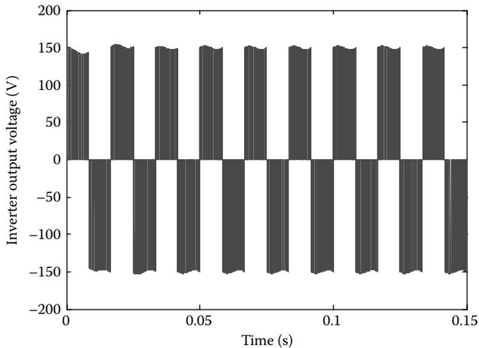
**FIGURE 1.56** Inverter output voltage for boost converter/inverter topology.
