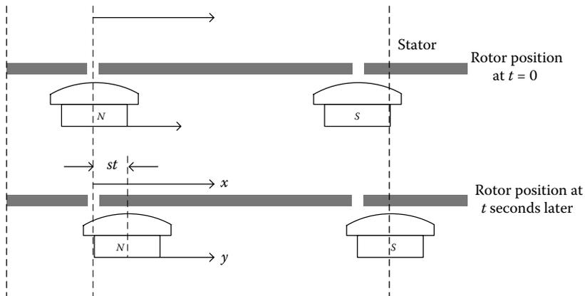
FIGURE 4.46 Coordinates and rotor position for stator winding.
