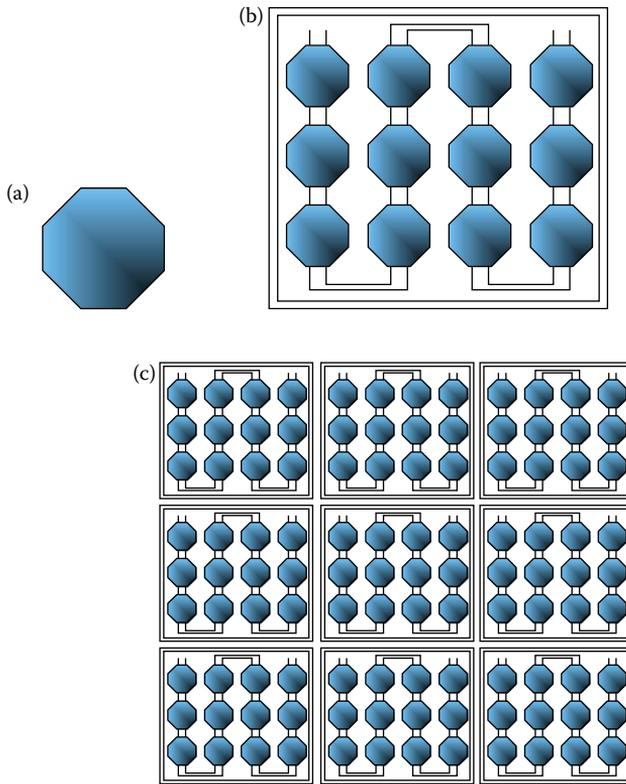
**FIGURE 1.2** (a) PV cell, (b) module, and (c) array.
