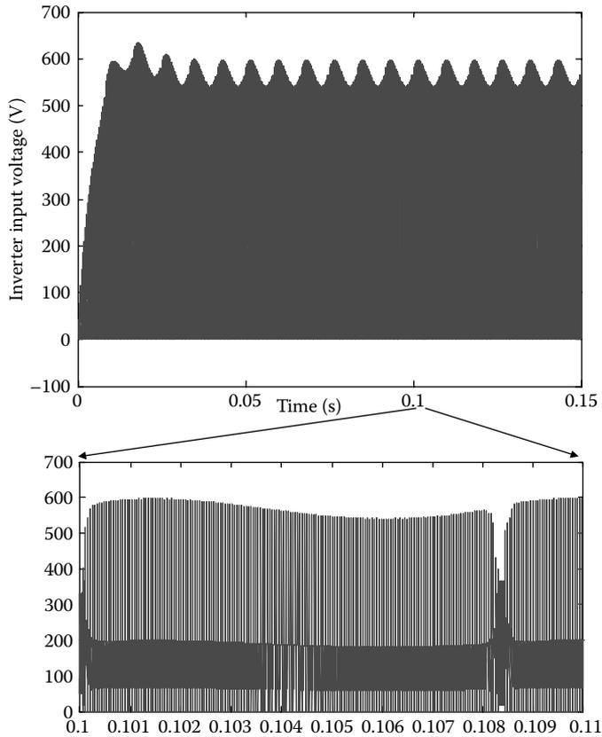
**FIGURE 1.48** Inverter input voltage in the fly-back converter.
