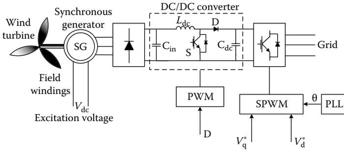
FIGURE 2.62 Synchronous generator with DC link regulation.
