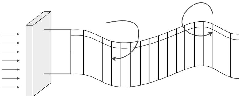
**FIGURE 4.60** Eel movement behind the bluff body.
