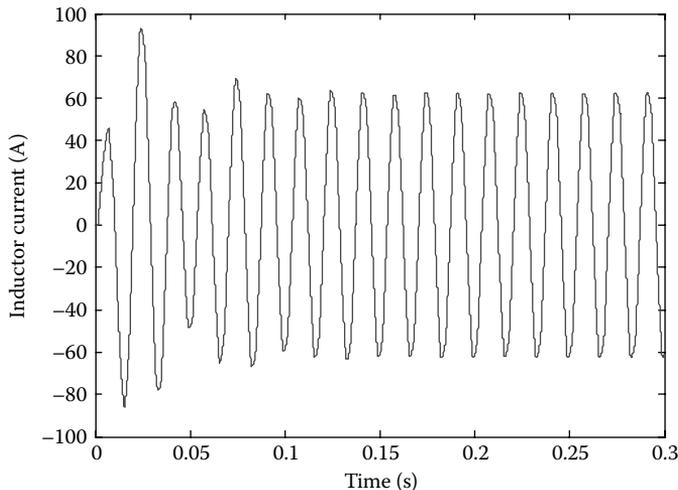
FIGURE 1.62 Output inductor current for an HBDC inverter.
