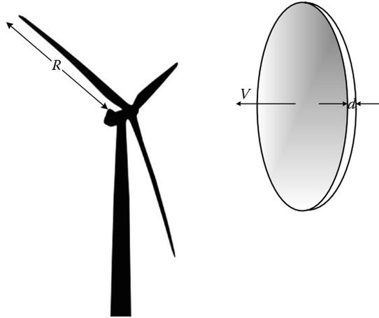
FIGURE 2.1 (See color insert following page 80.) Kinetic energy of wind.
