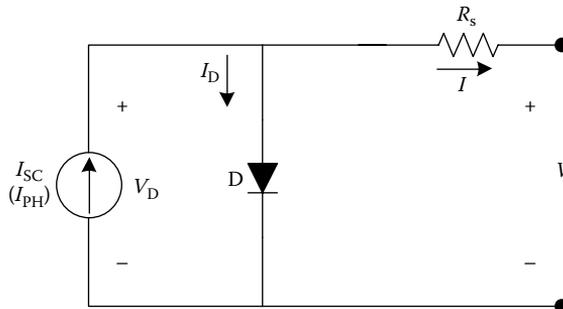
FIGURE 1.9 Model for a single solar cell.
