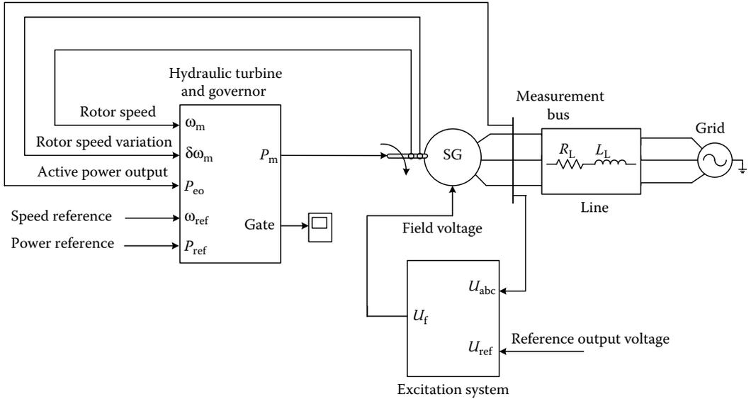
FIGURE 3.28 Hydraulic turbine and governor coupled to a synchronous generator.
