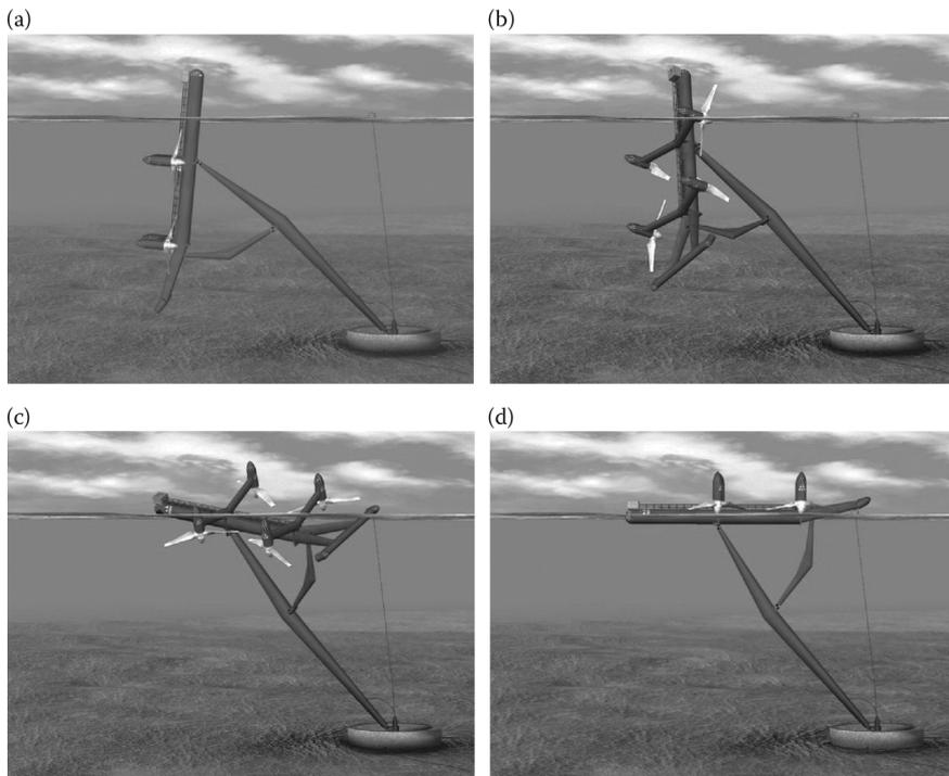
**FIGURE 3.47** (See color insert following page 80.) Position transformation of SST to its maintenance position. (a) Water is started to be pumped out of the main body, (b) swing arm started to roll, (c) rotors are rising to the water surface, (d) rotors reach a stable position on the sea surface. (Courtesy of Semi-Submersible Turbine, TidalStream Limited “*The Platform for Tidal Energy,*” available at: <http://www.tidalstream.co.uk/>)
