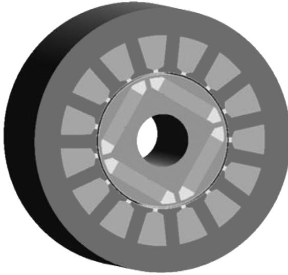
FIGURE 2.12 BLDC generator cross-sectional view (inner rotor type).
