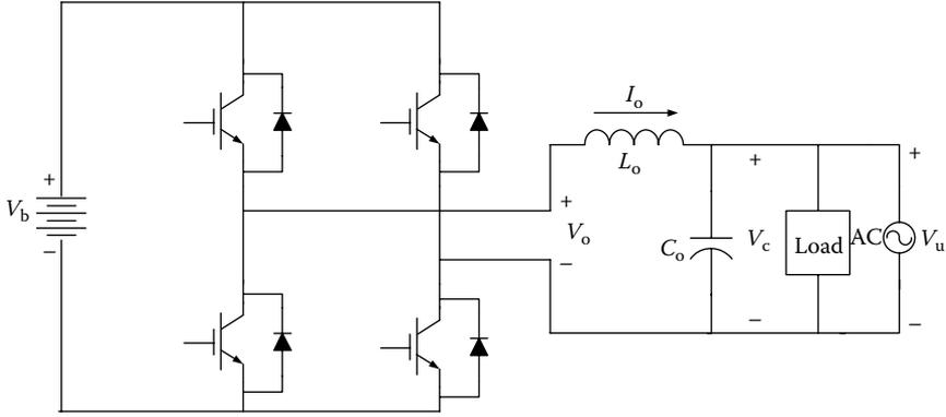
FIGURE 1.90 Bidirectional inverter/converter.
