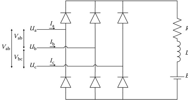
FIGURE 4.42 Three-phase diode rectifier schematic where a, b, and c are the linear generator phases.
