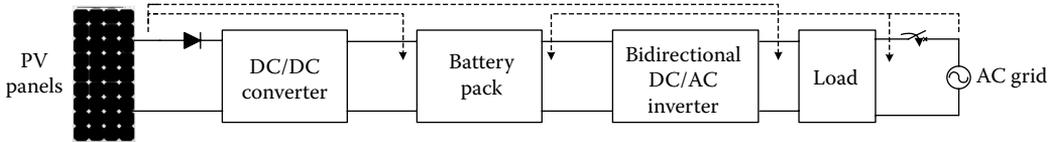
FIGURE 1.82 Operation mode 2 for the proposed residential system.
