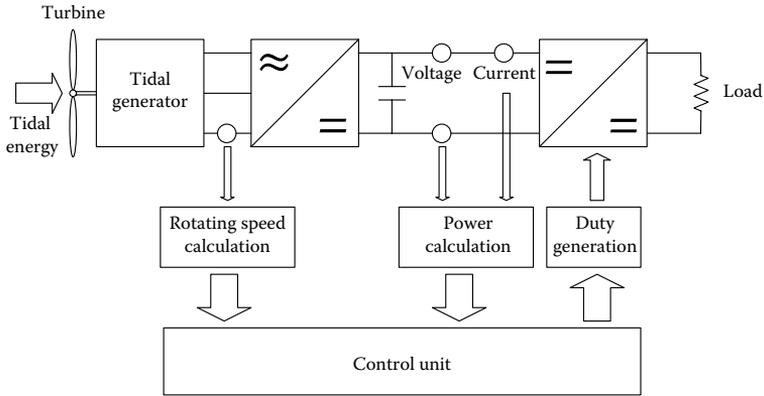
FIGURE 3.64 Control method based on current speed calculation.
