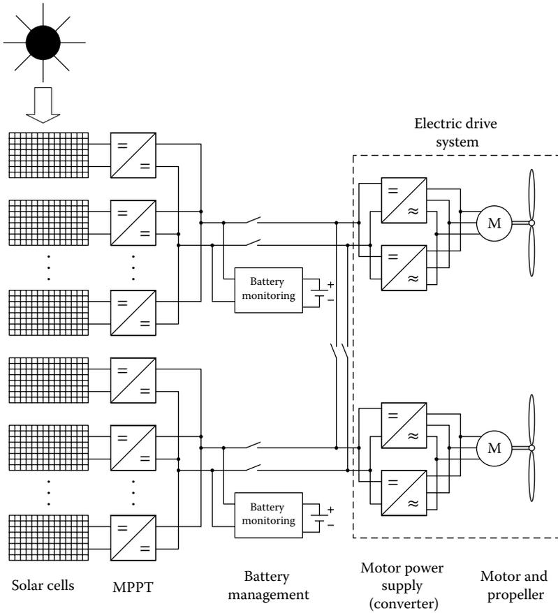
FIGURE 1.111 Electrical system of the proposed airplane.
