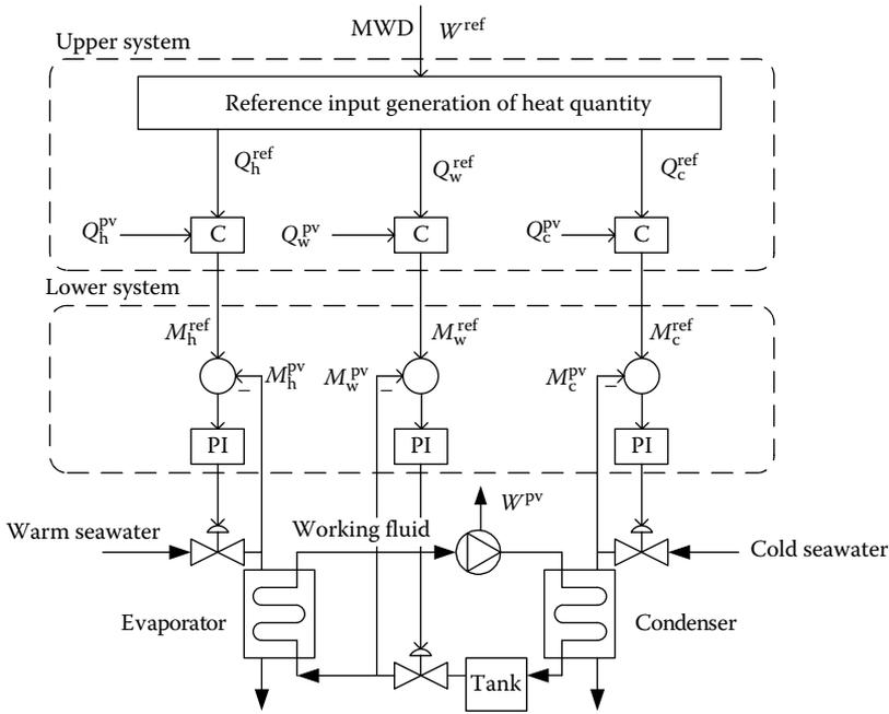
FIGURE 5.22 Block diagram of the OTEC system controller.
