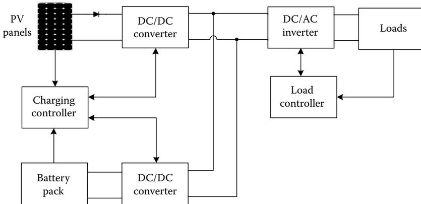
FIGURE 1.76 PV/battery connection—type 4.
