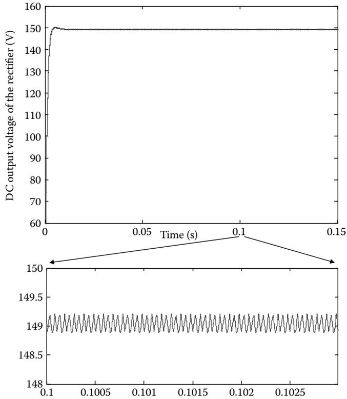
FIGURE 1.45 Output voltage of the push-pull converter.
