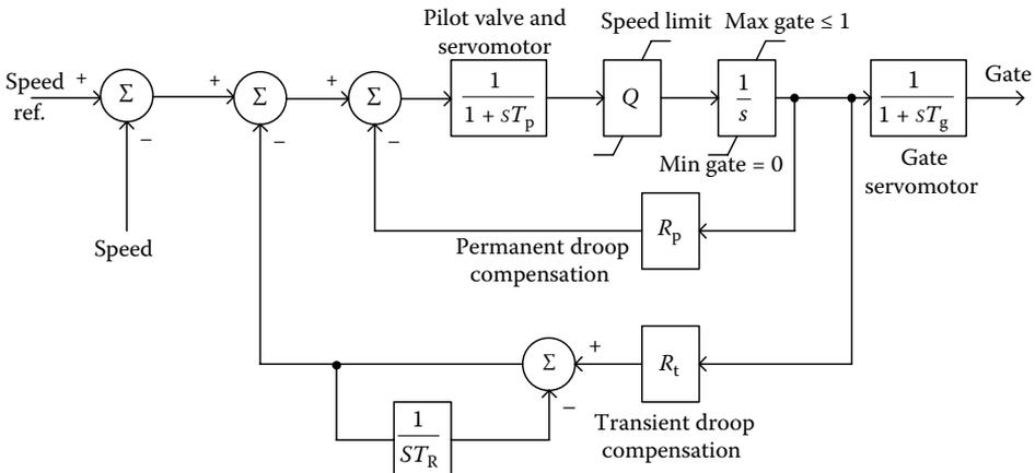
FIGURE 3.27 A typical hydro turbine governor model.
