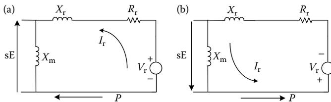
**FIGURE 2.41** Power transfer of DFIG by controlling the slip: (a) power transfer to DFIG and (b) power transfer from DFIG.
