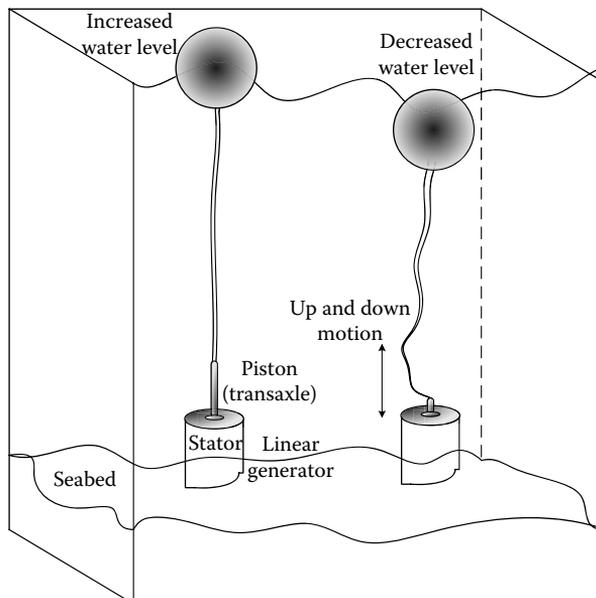
FIGURE 4.9 Linear generator–based buoy-type wave energy harvesting method.
