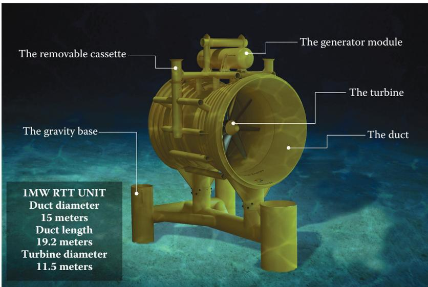
**FIGURE 3.44** A generating system with a horizontal axis turbine, Rotech Tidal Turbine. (Courtesy of Rotech Tidal Turbine (RTT), Lunar Energy™, Harnessing Tidal Power, available at: <http://www.lunarenergy.co.uk/>)
