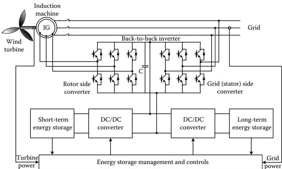
FIGURE 2.49 Multiple-level energy storage in DFIG system.
