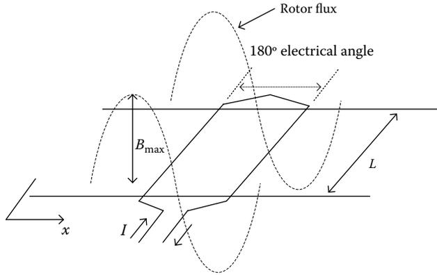
FIGURE 4.45 The traveling flux wave of stator winding.
