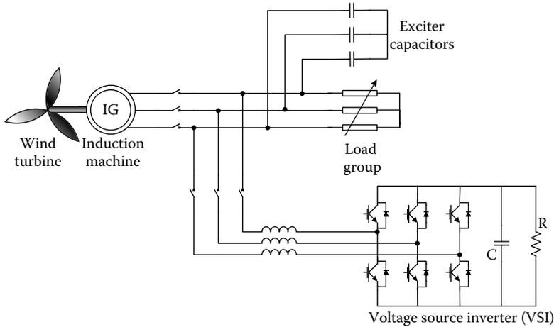
FIGURE 2.37 Induction generator controlled by VSI with exciter capacitors.
