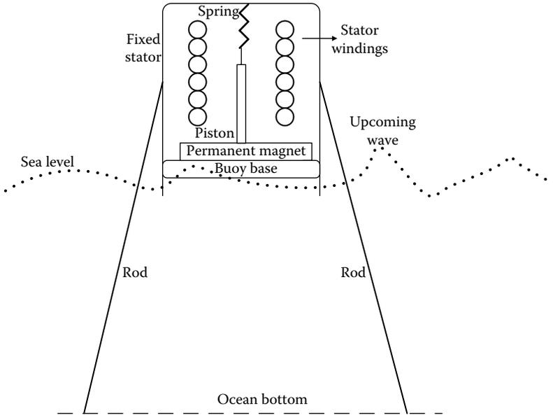
FIGURE 4.39 Schematic of an LFM used for WEC.
