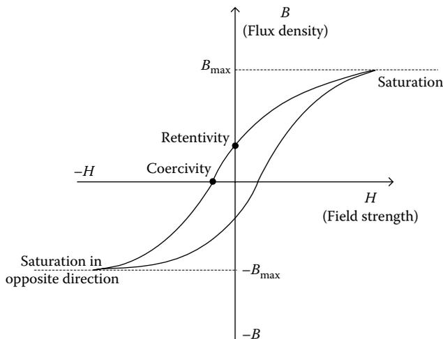
FIGURE 4.51 Flux density  $B$  versus field strength  $H$ .
