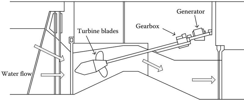
FIGURE 3.21 Tubular turbine.
