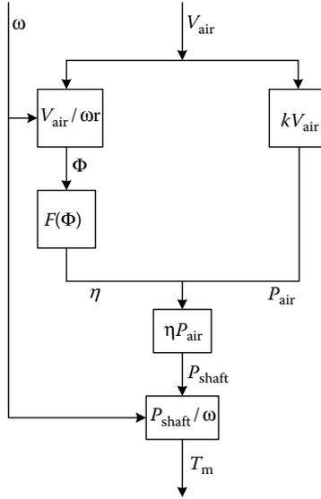
FIGURE 4.20 Block diagram of the Wells turbine.
