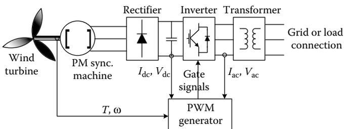
FIGURE 2.26 Block diagram of the simulated wind-turbine-driven PMMSG.
