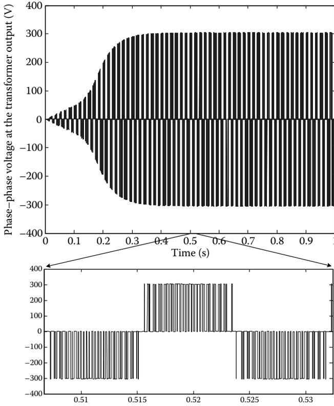
FIGURE 2.32 Phase-to-phase voltage at the transformer output.
