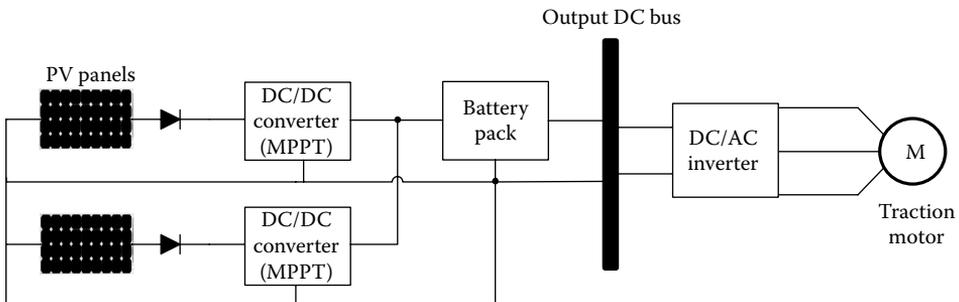
FIGURE 1.100 Distributed solar panel and power tracker configuration.
