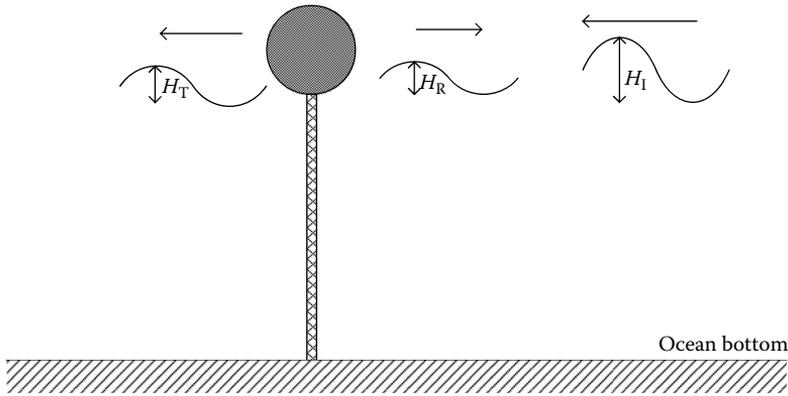
**FIGURE 4.6** Side view of a fixed body in waves showing incident, reflected and transmitted waves. (Modified from W.J. Jones and M. Ruane, "Alternative electrical energy sources for Maine, Appendix I, Wave Energy Conversion by J. Mays," Report No. MIT-E1 77-010, MIT Energy Laboratory, July 1977.)
