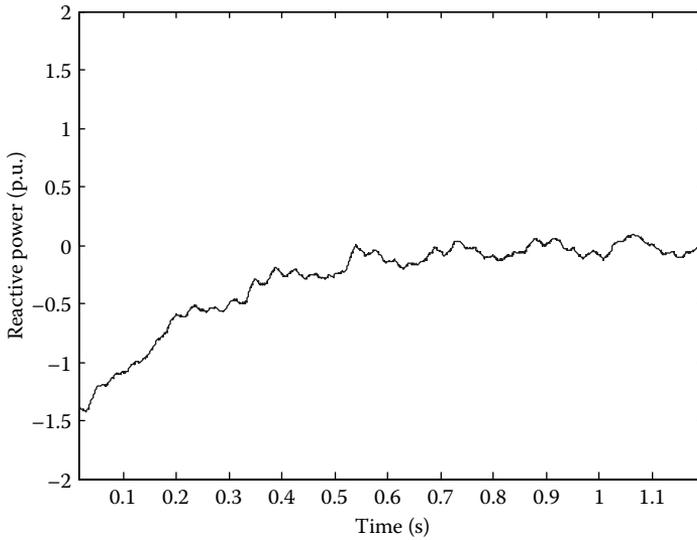
FIGURE 2.55 Reactive power output to the grid side.
