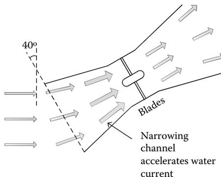
**FIGURE 3.45** Ducted turbine cross section.
