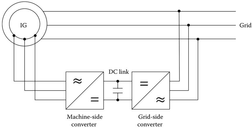
FIGURE 4.67 DFIG topology with back-to-back converters.
