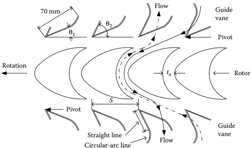
FIGURE 4.28 Impulse turbine with self-pitch-controlled guide vanes by link motion (ISGV).
