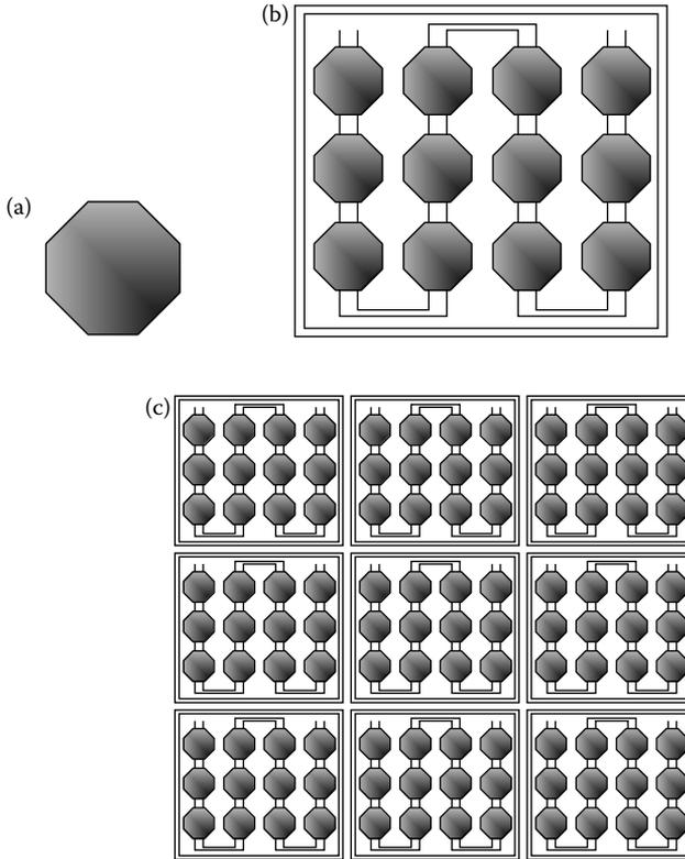
**FIGURE 1.2** (See color insert following page 80.) (a) PV cell, (b) module, and (c) array.
