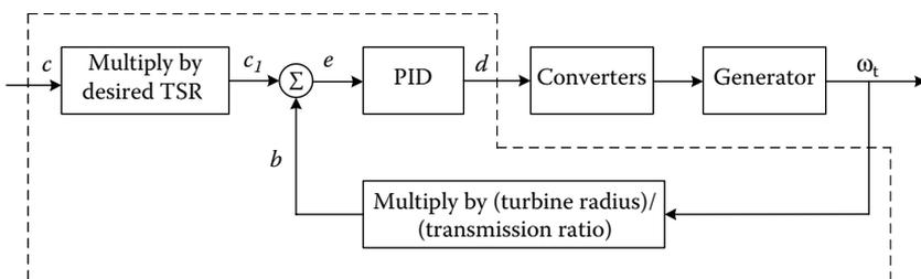
FIGURE 3.63 Block diagram of a MPPT controller.
