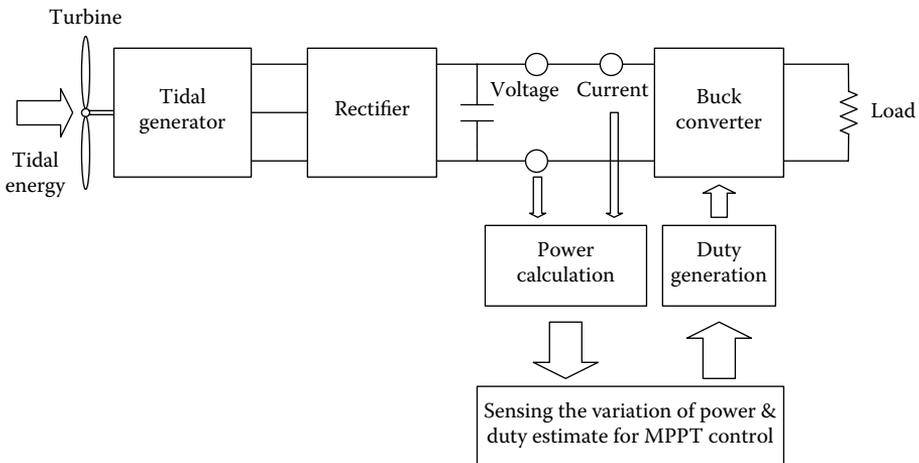
FIGURE 3.65 Block diagram of a MPPT control system.
