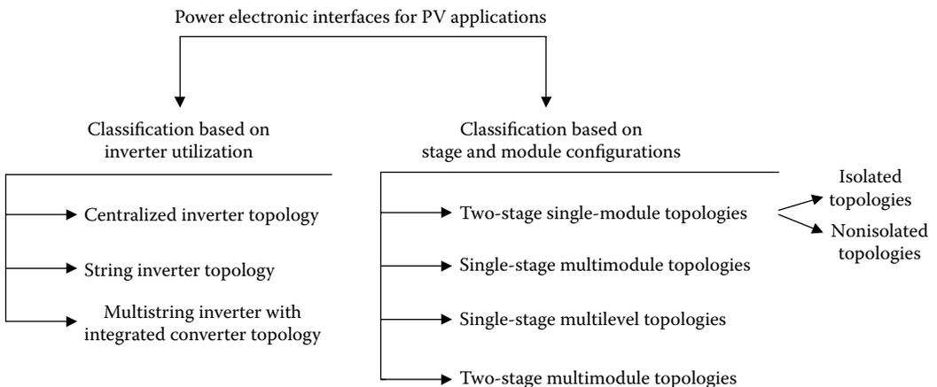
**FIGURE 1.38** Power electronic interfaces classification based on inverter utilization and stage/module configurations.
