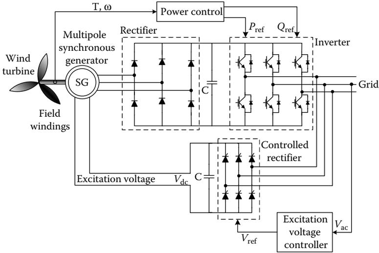
FIGURE 2.60 Multipole synchronous generator for wind turbine applications.
