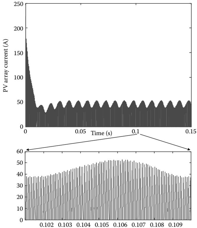
**FIGURE 1.47** PV array current of the fly-back converter.
