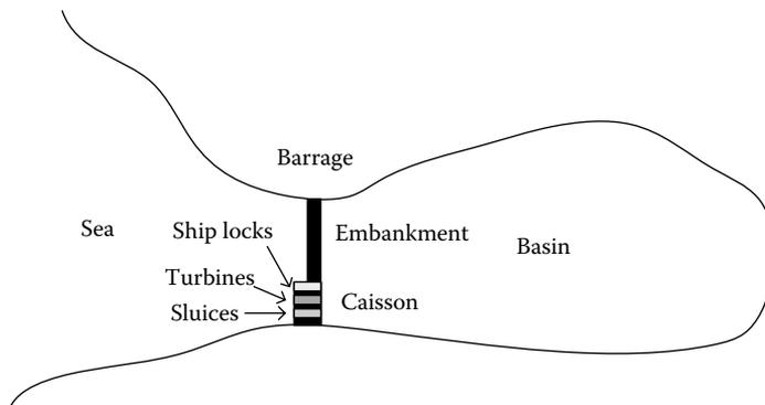
FIGURE 3.11 Barrage components.
