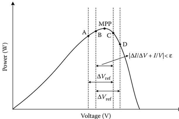
FIGURE 1.18 Operating point trajectory of incremental conductance–based MPPT.
