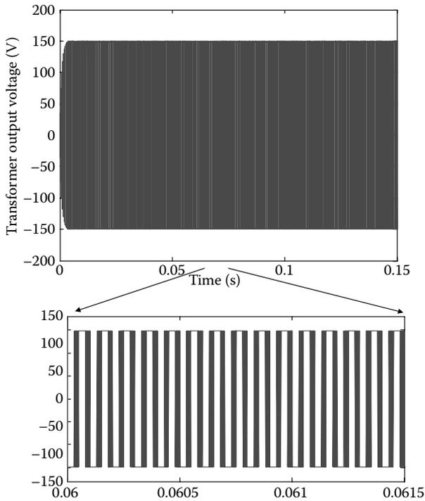
FIGURE 1.44 Transformer output voltage in the push-pull converter.
