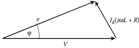
FIGURE 2.16 Back EMF and voltage phasor diagram.
