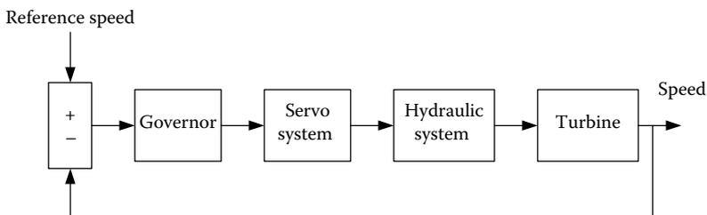
FIGURE 3.22 Hydro turbine speed control model.
