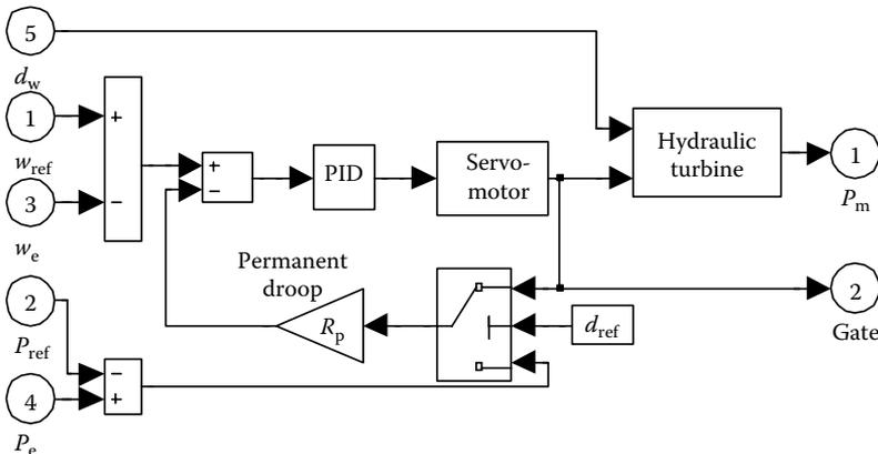
FIGURE 3.31 Complete turbine, governor, and servomotor model.
