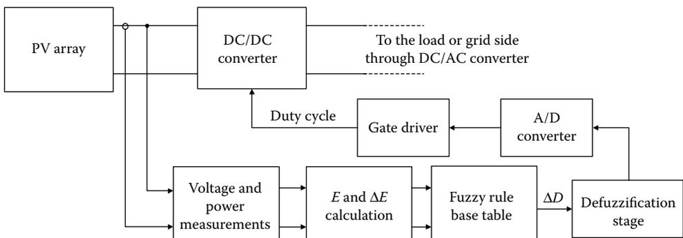
**FIGURE 1.27** Implementation of fuzzy logic controller-based MPPT.
