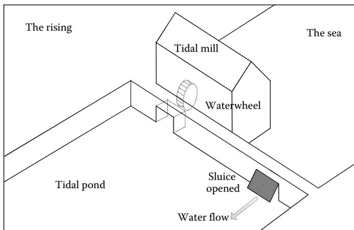
**FIGURE 3.4** Water flows inside to the tidal pond.
