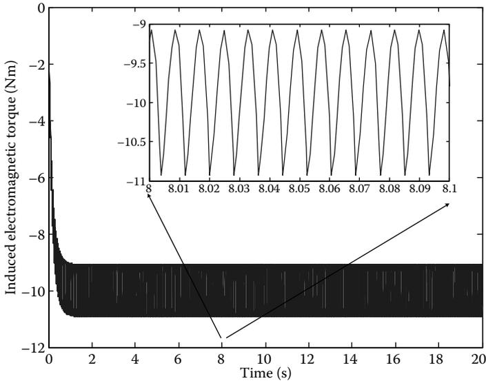
FIGURE 2.22 Electromagnetic torque induced by the BLDC generator.
