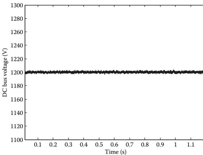
FIGURE 2.56 DC bus voltage between the converters.
