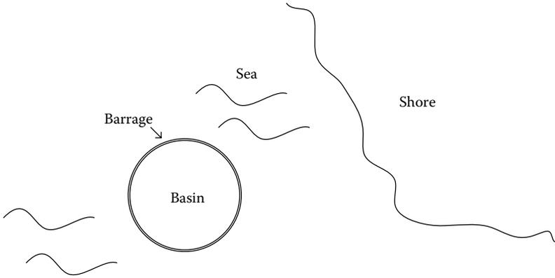
FIGURE 3.15 Schematic diagram of a tidal lagoon.
