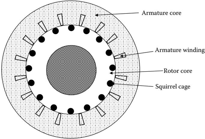
FIGURE 4.56 Cross-sectional view of induction machine structure.
