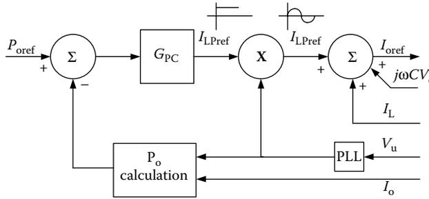
FIGURE 1.93 Block diagram of the power conditioner.
