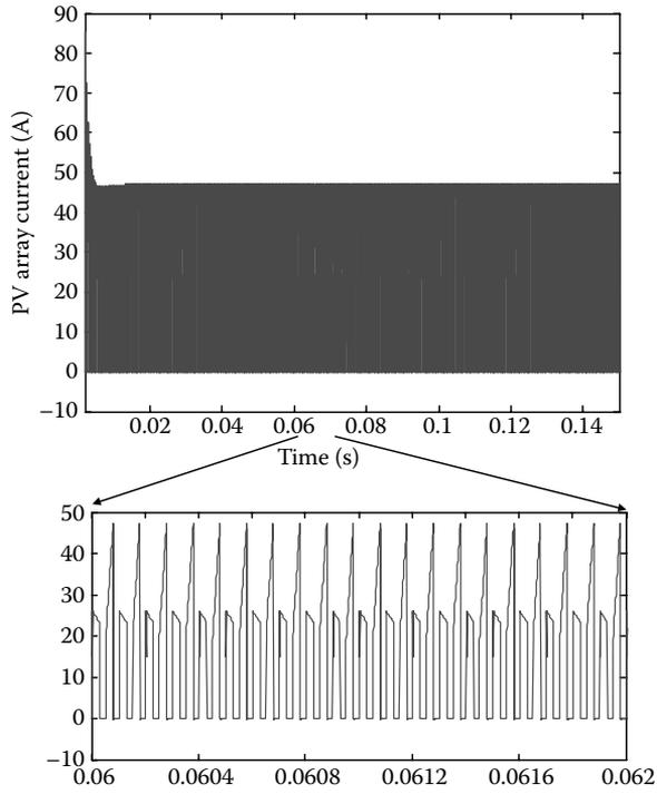
FIGURE 1.43 PV array current for push-pull converter.
