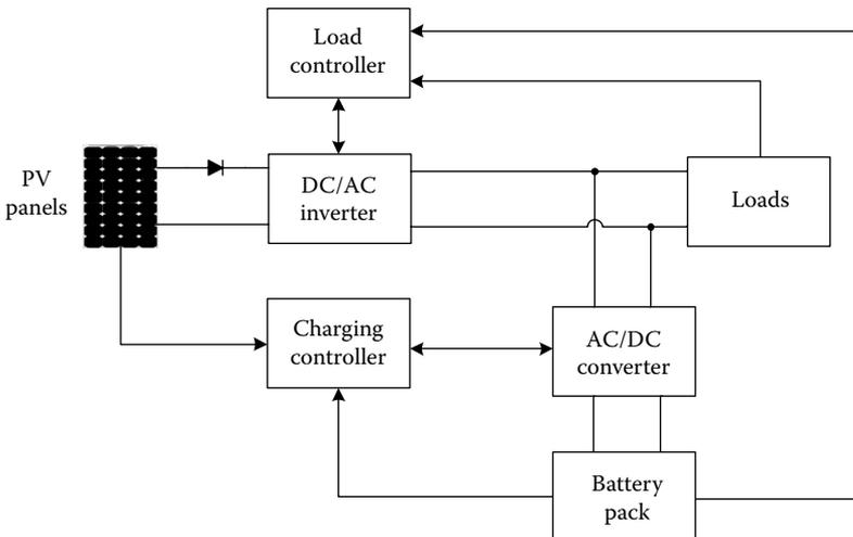
FIGURE 1.75 PV/battery connection—type 3.
