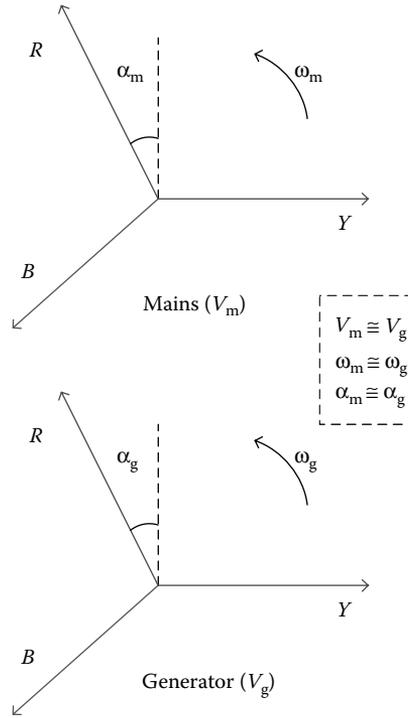
FIGURE 3.73 Phasor diagram for synchronized grid and generator.
