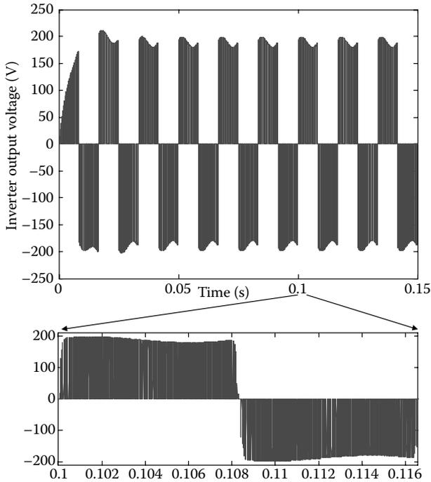
FIGURE 1.49 AC output voltage of the inverter.
