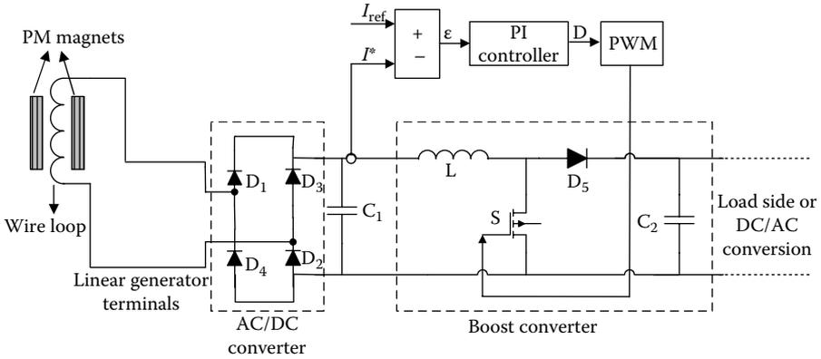
FIGURE 4.35 System-level configuration of the linear generator and power converters.
