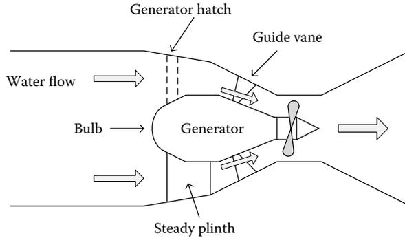
FIGURE 3.17 Bulb turbine.
