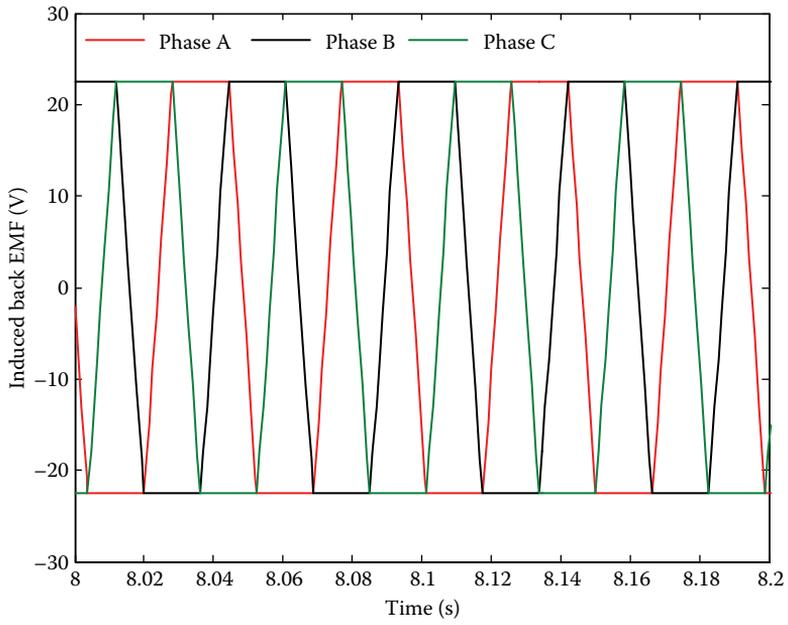
FIGURE 2.21 Back EMF induced by the BLDC phases.
