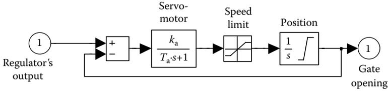
FIGURE 3.30 Servomotor model.
