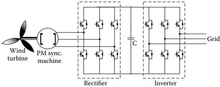
FIGURE 2.25 PMMSG with a back-to-back inverter.
