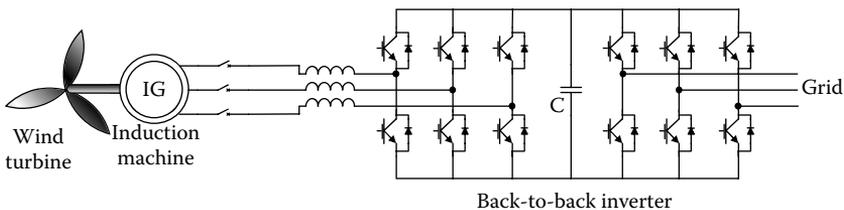
FIGURE 2.38 Induction machine controlled by a back-to-back inverter.
