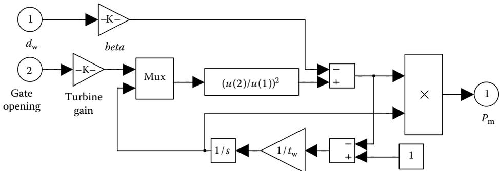
FIGURE 3.29 Hydraulic turbine model.
