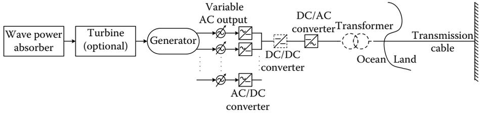
FIGURE 4.3 System-level diagram with the offshore transformer.
