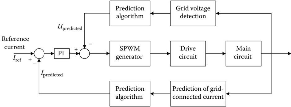
FIGURE 3.71 Control system of the inner control loop.
