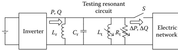
FIGURE 3.69 Islanding detection circuit.
