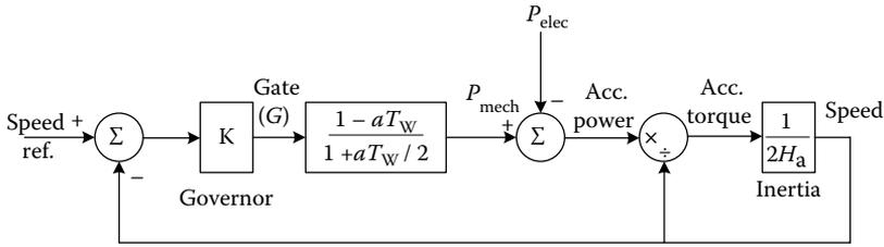
FIGURE 3.26 Hydro turbine and speed control linear model.
