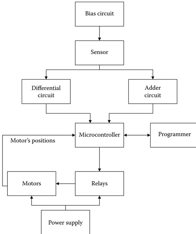
**FIGURE 1.15** Block diagram of the sensor output evaluation and motor control for sun tracker.
