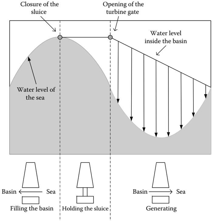
FIGURE 3.12 Process of the ebb generation approach.
