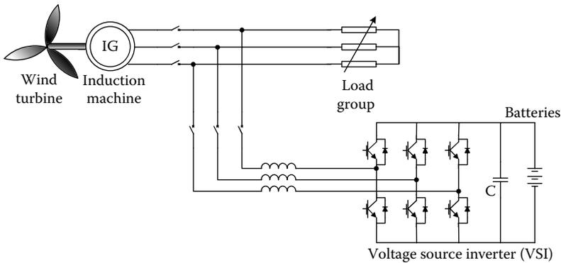
FIGURE 2.45 Voltage and frequency control using energy storage.
