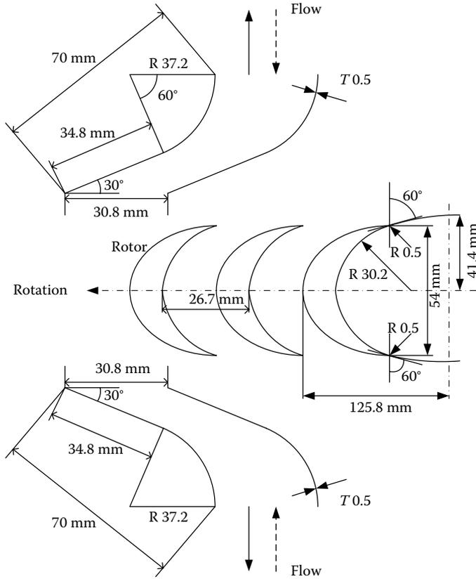
FIGURE 4.29 Impulse turbine with fixed guide vanes.
