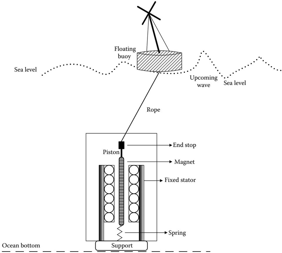
FIGURE 4.41 Another method of using LFMs for WEC.
