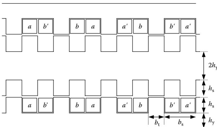
FIGURE 4.58 Linear switched reluctance machine cross-sectional view.
