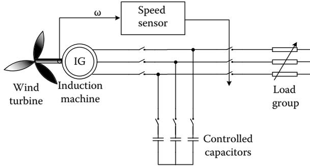
FIGURE 2.34 Conventional control scheme for the induction generator.
