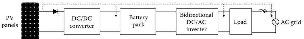
FIGURE 1.83 Operation mode 3 for the proposed residential system.
