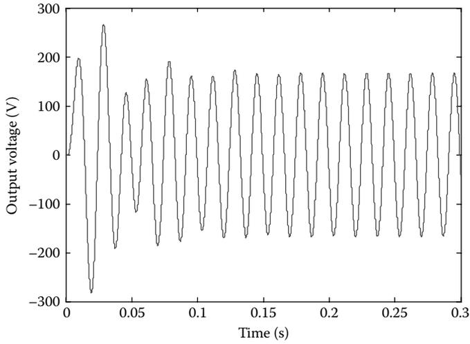
FIGURE 1.63 Output voltage for an HBDC inverter.
