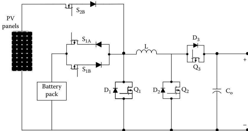
FIGURE 1.78 Positive output multiple input buck-boost converter.
