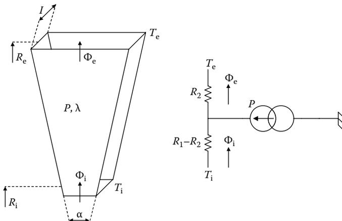
FIGURE 4.55 Unity volume and thermal equivalent circuit.
