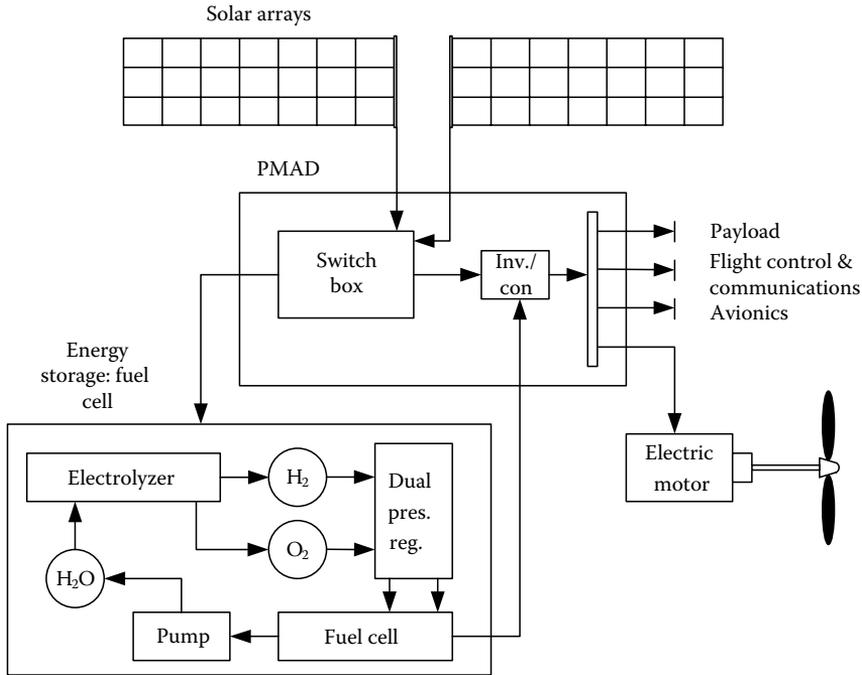
FIGURE 1.113 Power system of the solar-powered UAV.
