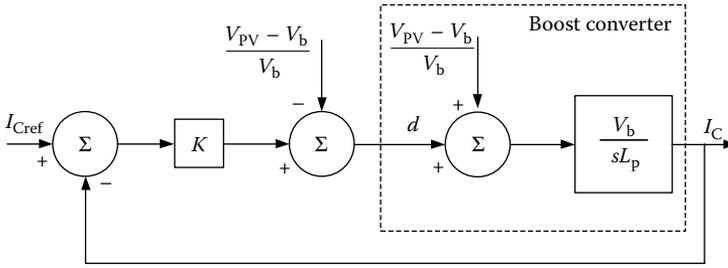
FIGURE 1.89 Current control scheme of the boost converter.
