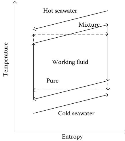
FIGURE 5.9 Comparison of mixture and pure fluid.
