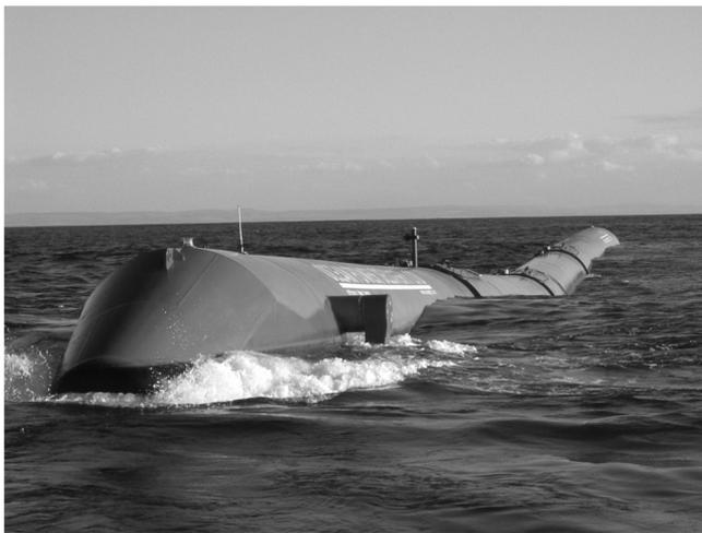
**FIGURE 4.72** (See color insert following page 80.) Pelamis WEC device at sea (Ocean Power Delivery Ltd). (Courtesy of R. Henderson, *Renewable Energy*, 31 (2), 271–283, 2006.)
