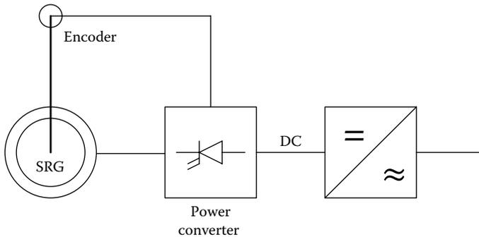
FIGURE 4.68 Overall grid connection diagram of an SRG.
