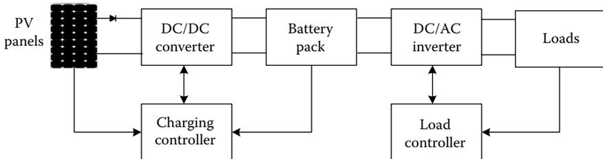
FIGURE 1.73 PV/battery connection—type 1.
