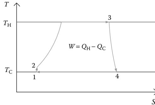
FIGURE 5.8 Temperature–entropy diagram for a Rankine cycle.
