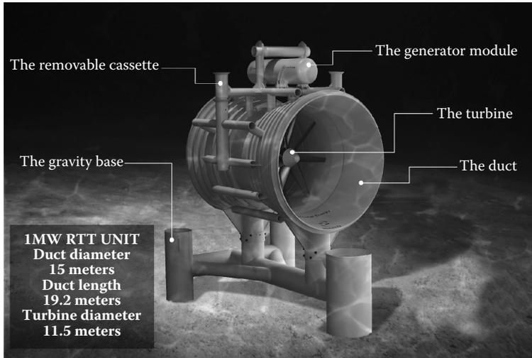
**FIGURE 3.44** (See color insert following page 80.) A generating system with a horizontal axis turbine, Rotech Tidal Turbine. (Courtesy of Rotech Tidal Turbine (RTT), Lunar Energy™, Harnessing Tidal Power, available at: <http://www.lunarenergy.co.uk/>)
