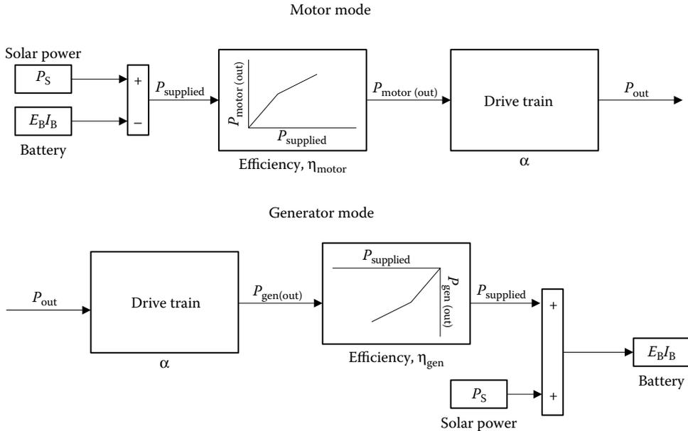
FIGURE 1.102 Power flow diagram in a solar EV.
