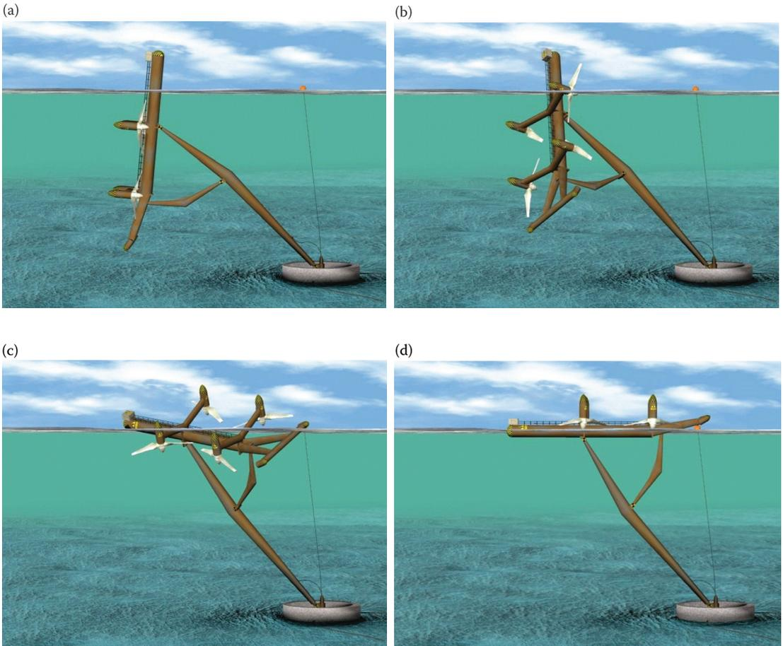
**FIGURE 3.47** Position transformation of SST to its maintenance position. (a) Water is started to be pumped out of the main body, (b) swing arm started to roll, (c) rotors are rising to the water surface, (d) rotors reach a stable position on the sea surface. (Courtesy of Semi-Submersible Turbine, TidalStream Limited “*The Platform for Tidal Energy,*” available at: <http://www.tidalstream.co.uk/>)
