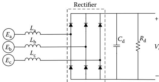
FIGURE 2.14 Diode rectifier connected to a BLDC generator.
