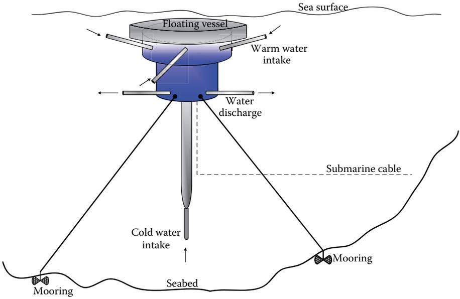
FIGURE 5.2 An offshore OTEC application.
