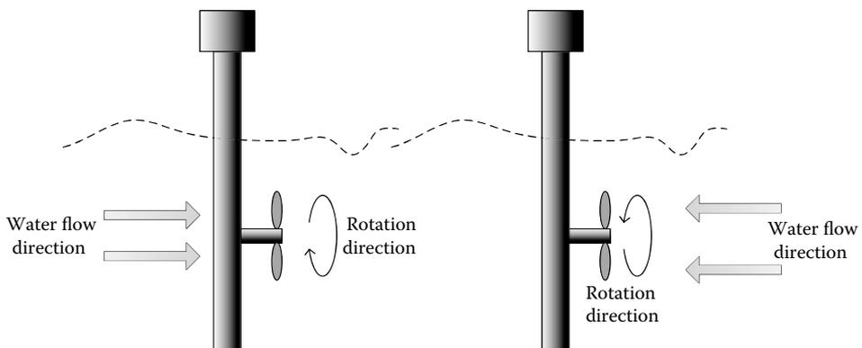
**FIGURE 3.49** Operation of a bidirectional horizontal axis turbine.
