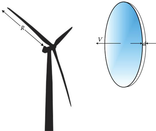
**FIGURE 2.1** Kinetic energy of wind.
