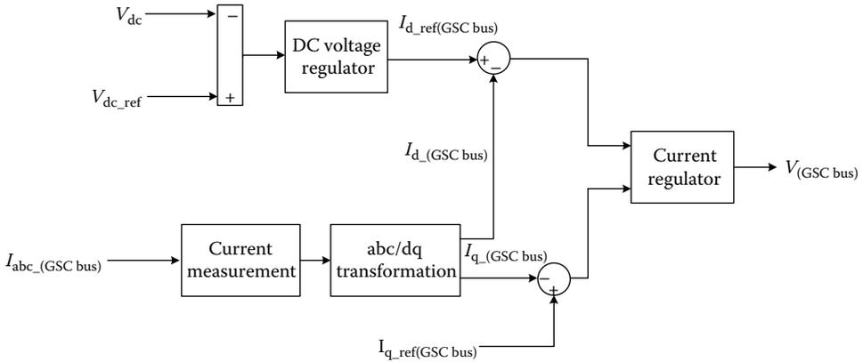
FIGURE 2.53 Block diagram of the GSC controller.
