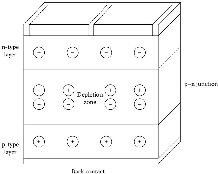
FIGURE 1.1 p–n junction of the PV cell.
