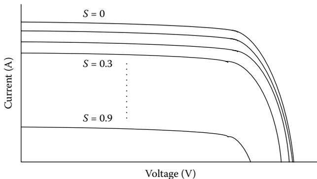
FIGURE 1.35  $I$ - $V$  characteristics under different shading conditions.
