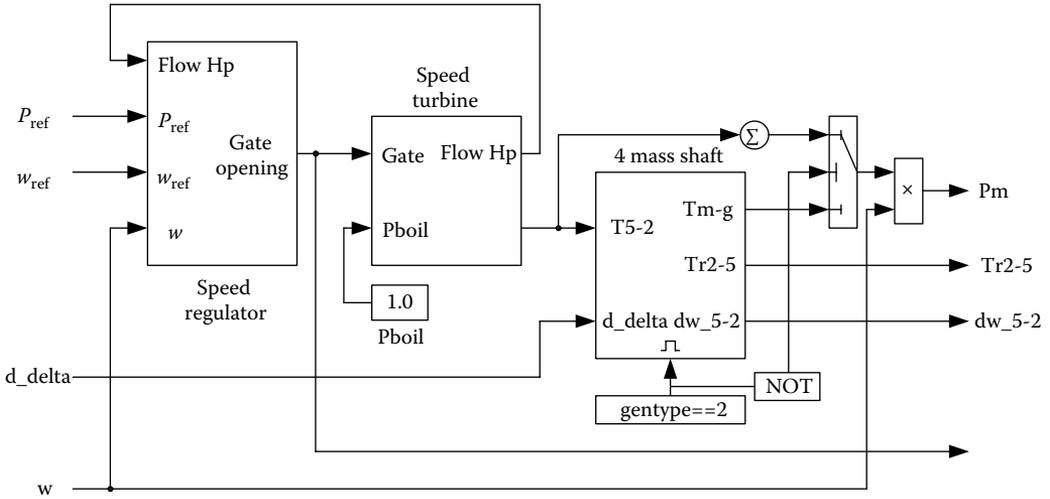
FIGURE 5.28 Complete governor, steam turbine, and shaft model.
