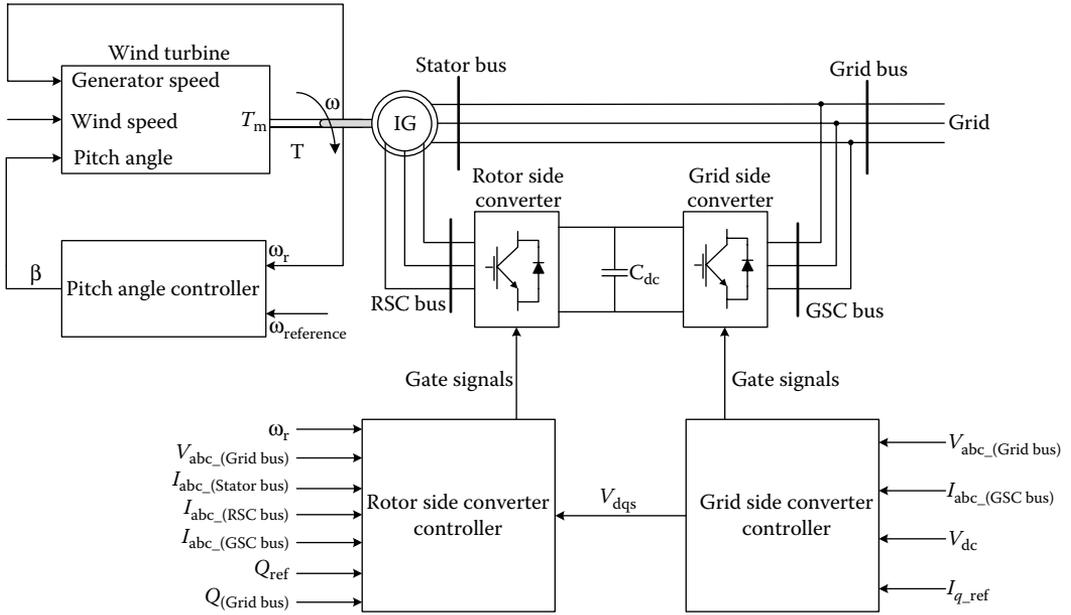
FIGURE 2.50 Block diagram of a DFIG topology.
