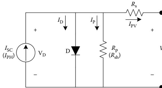
FIGURE 1.7 Single-diode model of solar cell equivalent circuit.
