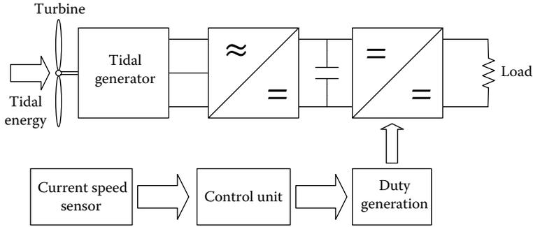
FIGURE 3.62 Control method based on current speed measurements.
