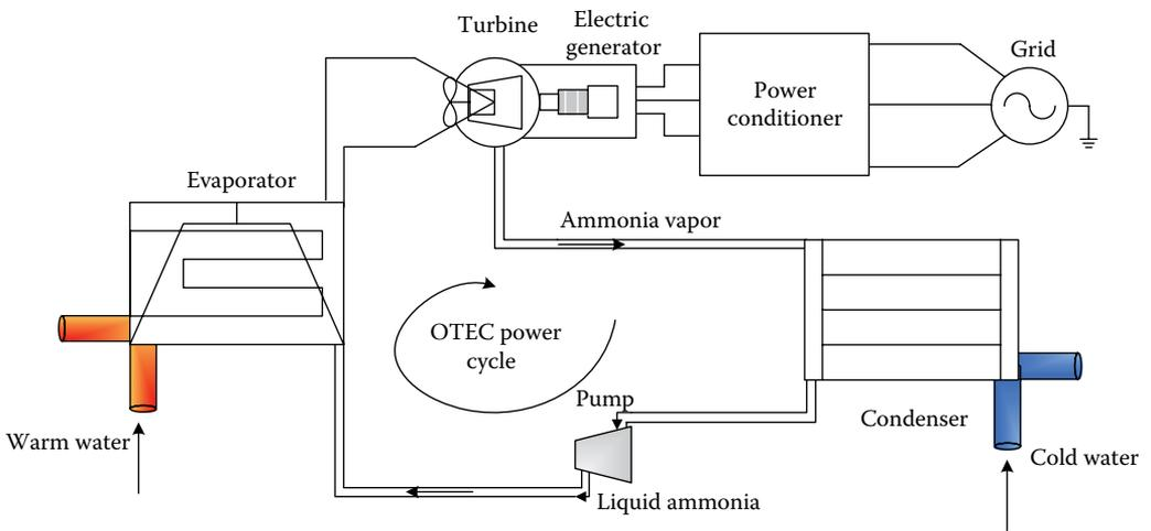
**FIGURE 5.1** A general overview of an OTEC system.
