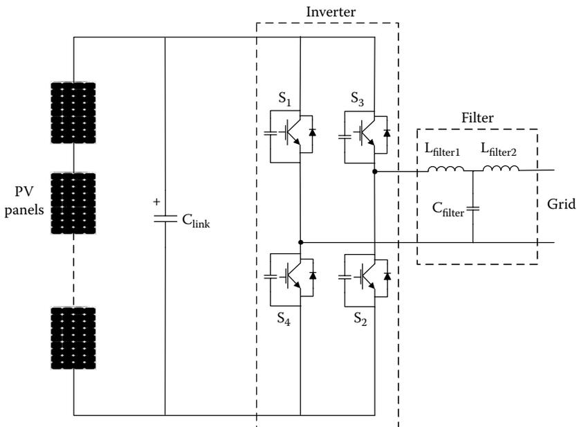
FIGURE 1.58 Single-stage inverter for multiple modules.
