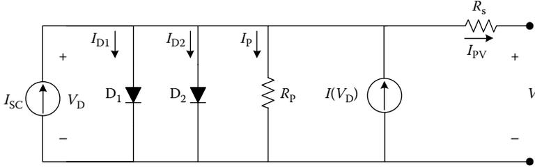
FIGURE 1.8 Dual-diode model.
