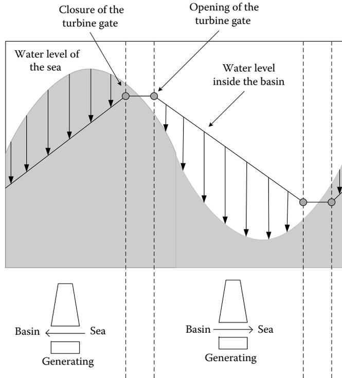
FIGURE 3.14 Process of the two-way generation approach.
