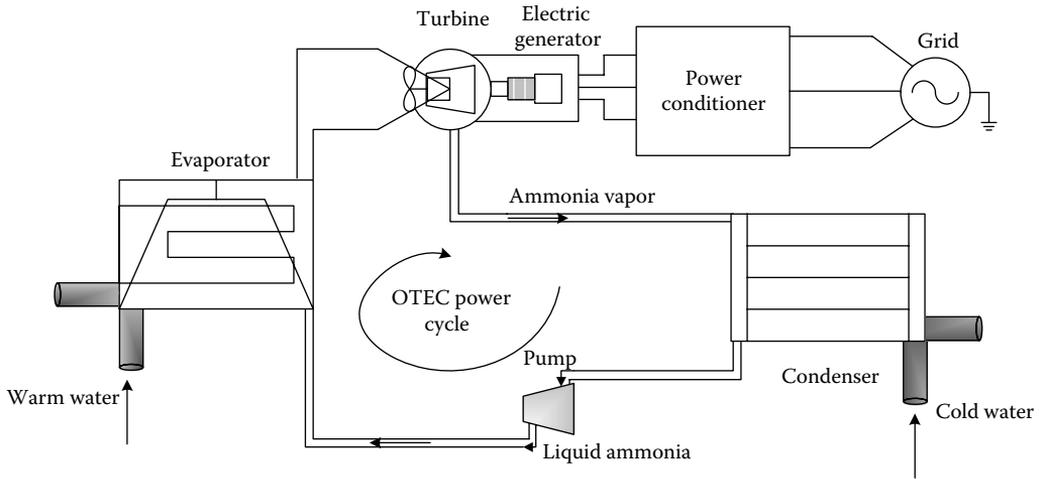
**FIGURE 5.1** (See color insert following page 80.) A general overview of an OTEC system.
