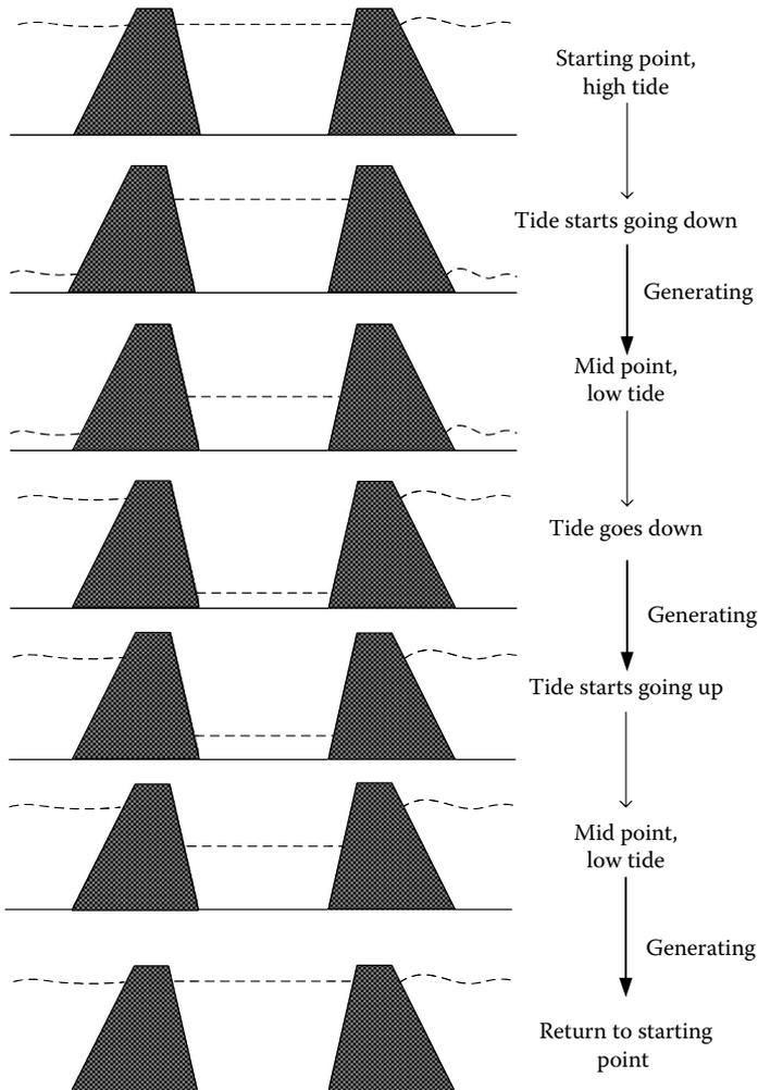
FIGURE 3.16 Operation process of a tidal lagoon.
