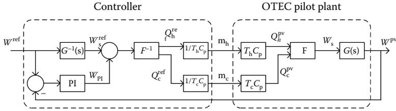
FIGURE 5.23 OTEC pilot model and controller structure.
