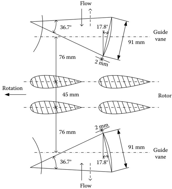
FIGURE 4.27 Biplane wells turbine with guide vanes.
