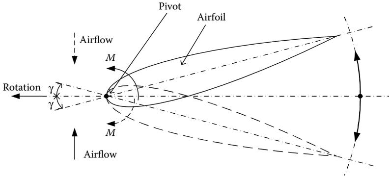
FIGURE 4.23 Turbine using self-pitch-controlled blades for WEC.
