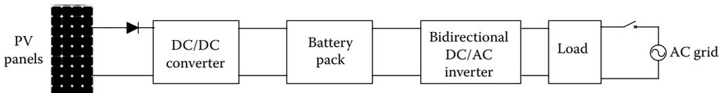
FIGURE 1.80 Power circuit of a residential PV system.
