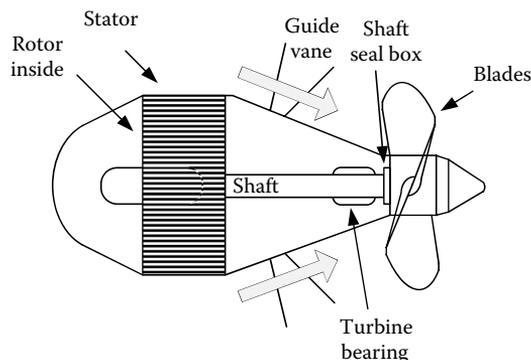
FIGURE 3.18 Bulb turbine inside.
