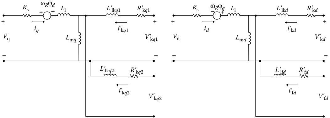
FIGURE 2.59 Synchronous machine  $q$ - and  $d$ -axis equivalent electrical circuits.
