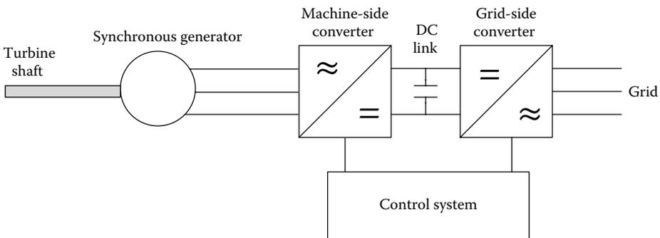
FIGURE 3.54 Variable speed operation of a synchronous generator.
