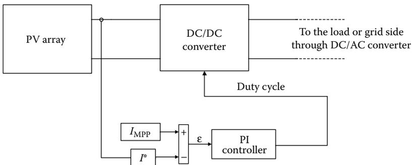
FIGURE 1.25 Implementation of fractional short-circuit-based MPPT.
