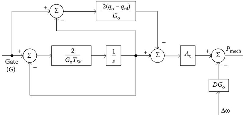
FIGURE 3.25 Linearized turbine model.
