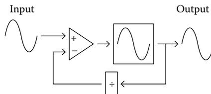
FIGURE 3.68 A simplified PLL principle.
