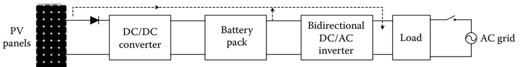
FIGURE 1.84 Operation mode 4 for the proposed residential system.
