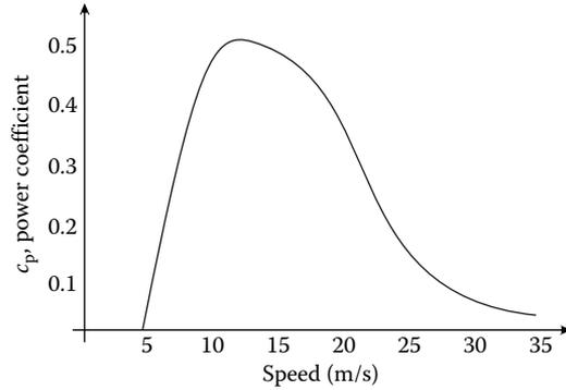
FIGURE 2.8 Power coefficient curve of a wind turbine.
