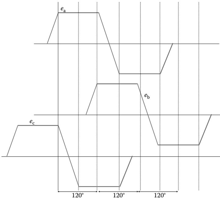
FIGURE 2.13 Induced EMF of a three-phase BLDC generator.
