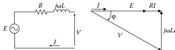
FIGURE 4.54 Electrical phasor diagram for  $\psi = 0$ .
