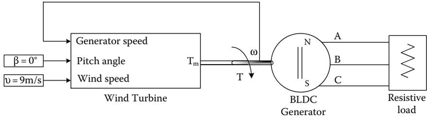
FIGURE 2.20 Block diagram of a wind turbine with a BLDC generator.
