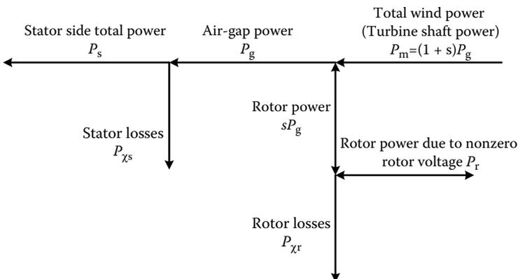
**FIGURE 2.44** Total power and power flow of DFIG.
