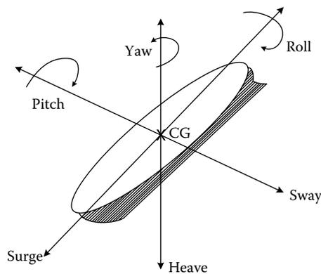
**FIGURE 4.7** Directions of motion of a floating body. (Modified from W.J. Jones and M. Ruane, "Alternative electrical energy sources for Maine, Appendix I, Wave Energy Conversion by J. Mays," Report No. MIT-E1 77-010, MIT Energy Laboratory, July 1977.)
