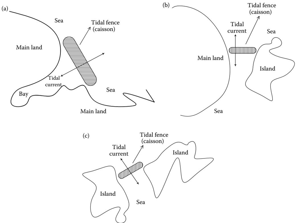
FIGURE 3.2 Tidal fences can be mounted (a) at the entrance of bays, (b) between the main land and an island, and (c) between two islands.
