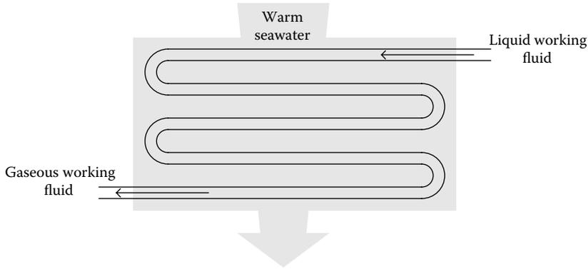
FIGURE 5.15 Schematic diagram of an evaporator.
