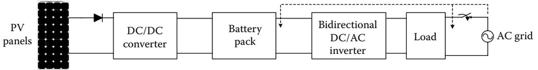
FIGURE 1.81 Operation mode 1 for the proposed residential system.
