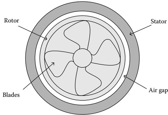
FIGURE 3.19 Generator structure of a rim turbine.
