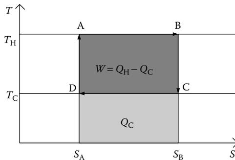
FIGURE 5.6 Temperature–entropy diagram for an ideal Carnot cycle.
