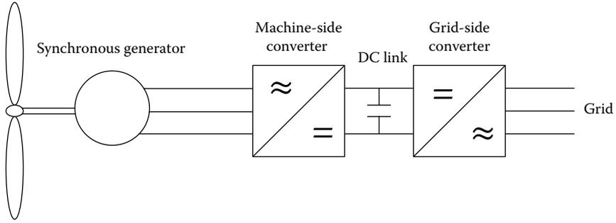
FIGURE 3.59 Variable-speed direct-driven (gearless) turbine.
