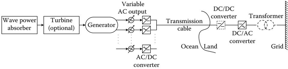
FIGURE 4.1 System-level diagram of ocean wave energy harvesting.
