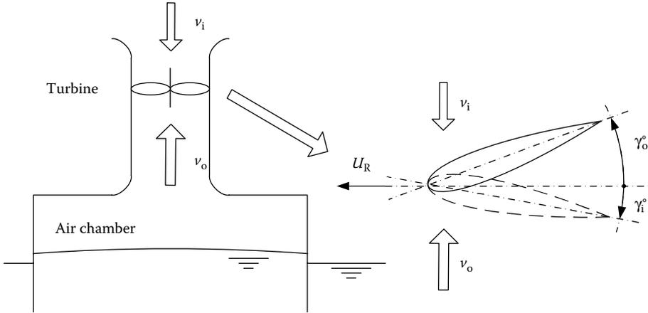
FIGURE 4.24 Overall view of wave energy turbine with self-pitch-controlled blades.
