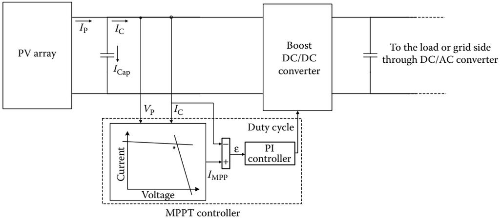
FIGURE 1.23 Linearized  $I$ - $V$  characteristics-based MPPT controller.
