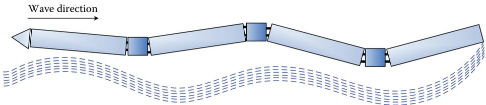
**FIGURE 4.73** General layout of the Pelamis WEC device.
