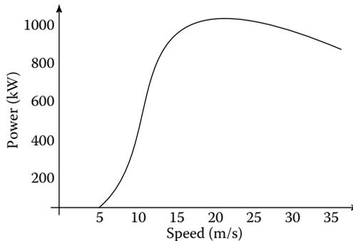
FIGURE 2.6 The power curve for a wind turbine.
