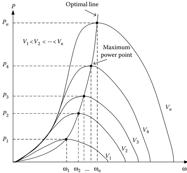
FIGURE 3.61 Generator power curves at various tidal speeds.
