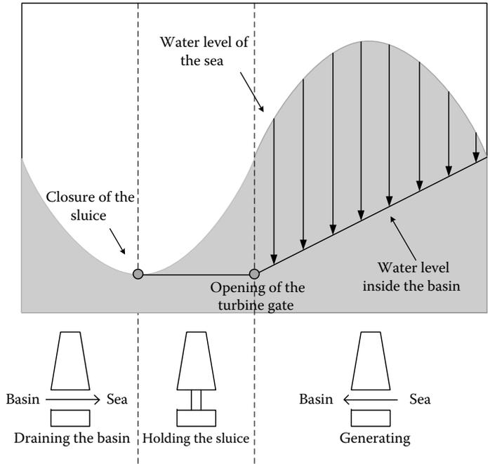
FIGURE 3.13 Process of the flood generation approach.
