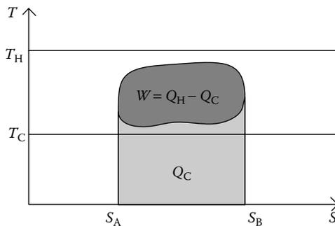
FIGURE 5.7 Temperature–entropy diagram for a generalized thermodynamic cycle.
