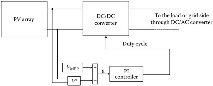
FIGURE 1.24 Implementation of fractional open-circuit-based MPPT.
