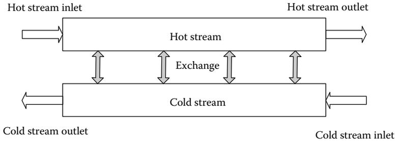
FIGURE 5.13 Countercurrent exchange.
