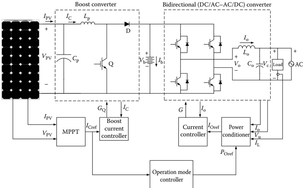
FIGURE 1.86 System configuration of the grid connected PV system.
