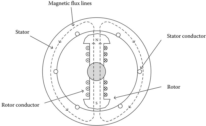
FIGURE 3.51 Conceptual representation of a two-pole synchronous machine.
