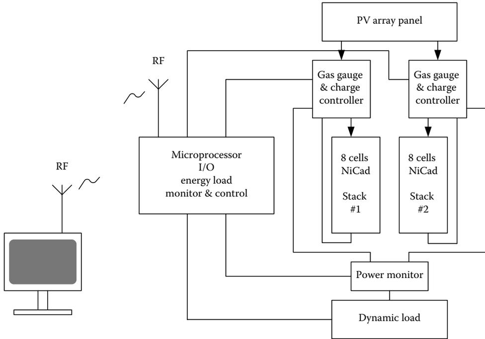
FIGURE 1.105 Solar energy system test-bed block diagram.
