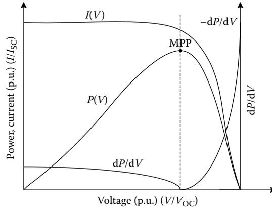
FIGURE 1.19 Normalized IV, PV, and  $|dP/dV|$  characteristics of a PV array.
