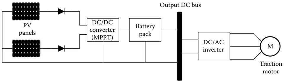
FIGURE 1.99 Block diagram of a solar EV.
