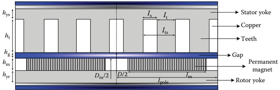
FIGURE 4.53 Cross-sectional view of two poles of the generator.
