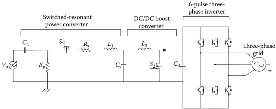
FIGURE 4.71 Power electronic interface schematic for piezoelectric/electrostrictive generators.
