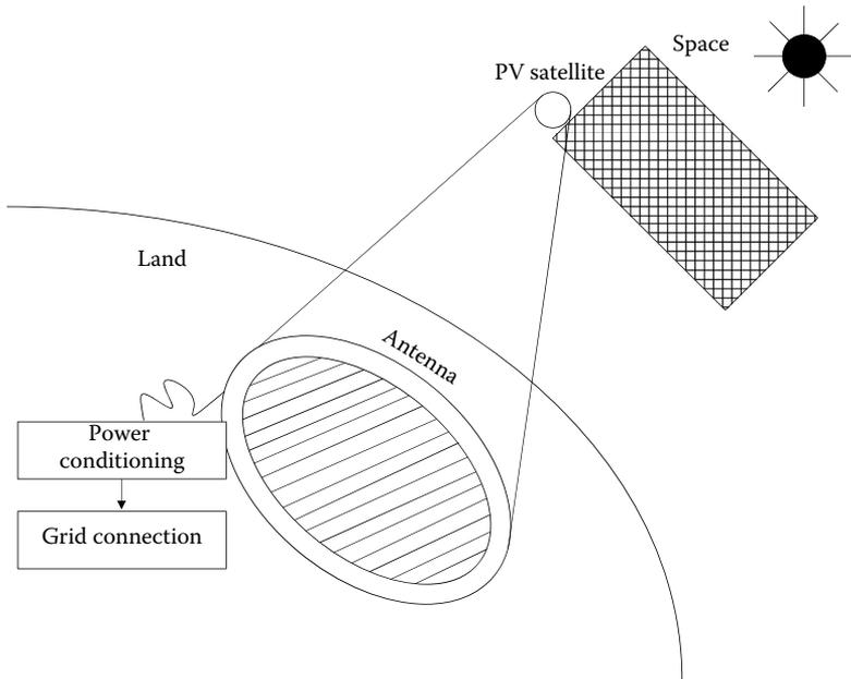
FIGURE 1.108 Concept of the solar power satellite system.
