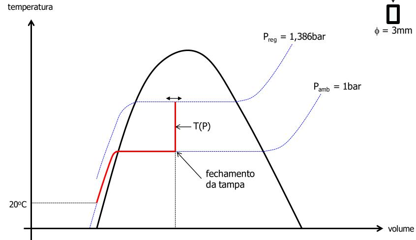
$$P_{reg} = \frac{9.8 \,\text{m/s}^2 \times 0.1 \,\text{kg}}{\pi \times (3 \cdot 10^{-3} \,\text{m})^2 / 4}$$
