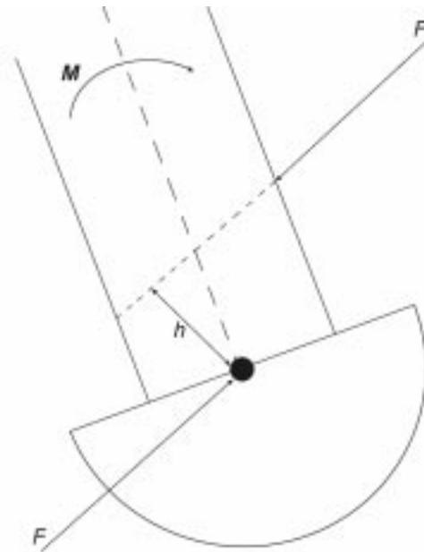
1.4 Free body diagram to calculate external forces and moments – the joint shown in Fig. 1.3 has been 'disarticulated' so that the forces acting on a single component can be analysed.
