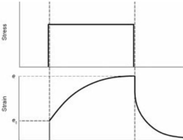
1.9 Illustration of viscoelastic behaviour. Note that when a stress is applied instantaneously, there is a time delay in the resulting strain. The same effect occurs when the stress is removed.
