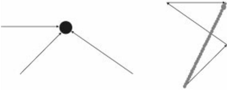
1.1 Summation of force vectors acting on a particle – vectors are added 'head to tail'. Resultant vector is from first tail to final head.
