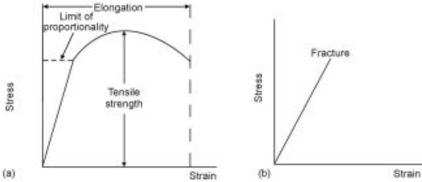
1.8 (a) Stress–strain diagram showing ductile behaviour in a tensile test. (b) Brittle behaviour in which fracture occurs before yield, i.e. there is no limit of proportionality.
