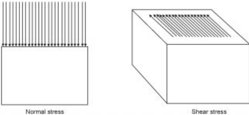
1.7 Diagram illustrating applied direct and shear stresses applied to a surface.
