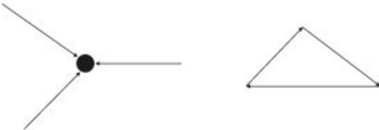
1.2 Equilibrium of force vectors – the rules for addition are identical to those in Fig. 1.1. However, in this situation the end point of the vector addition coincides with the start point so that there is zero net resultant.
