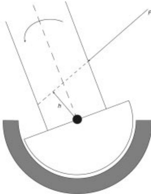
1.3 Moment produced by a force acting at a distance from the centre of rotation – note that the moment is equal to the magnitude of force  $F$  and the perpendicular distance  $h$ .
