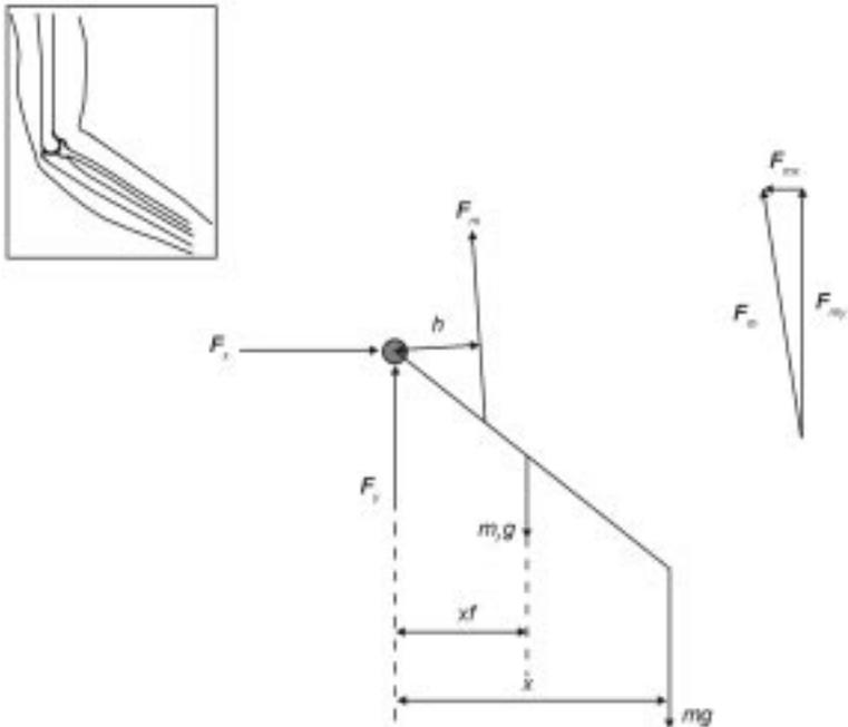
1.5 Free body diagram of forearm when supporting a hand-held weight. Note the force vectors representing the weight carried and the weight of the forearm. The vector triangle illustrates how the muscle force line of action may be broken down into two components corresponding with the coordinate axes.
