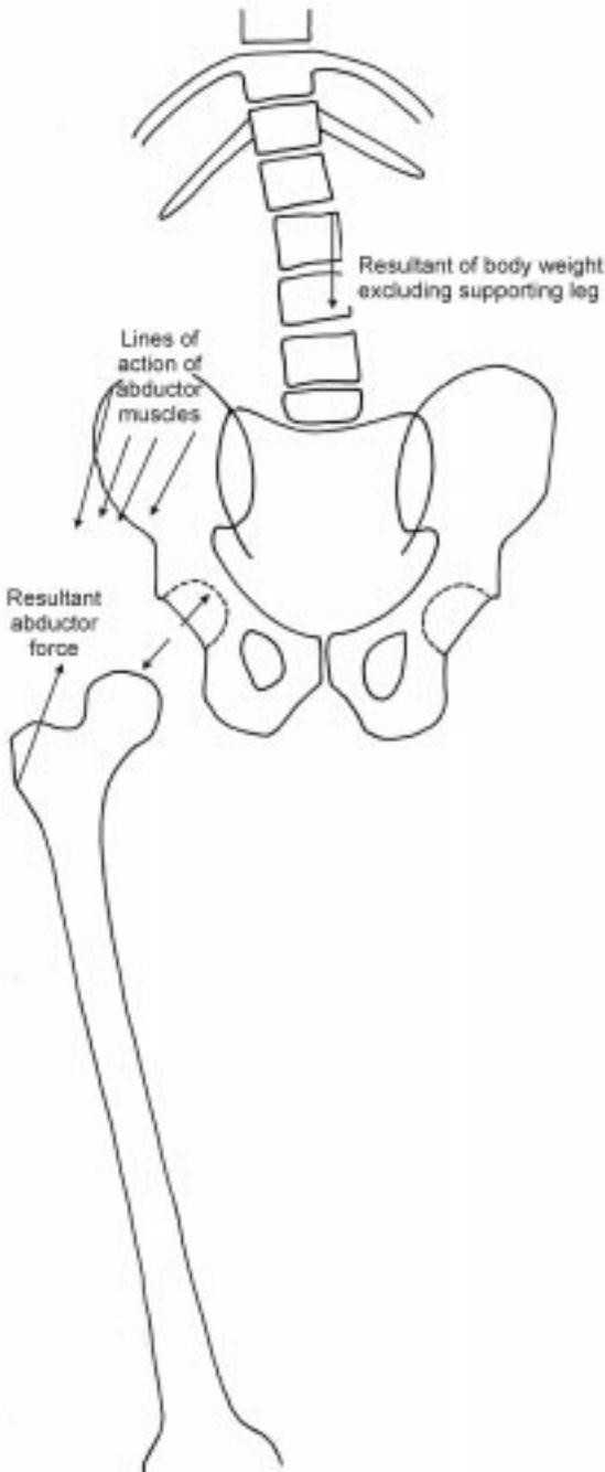
1.6 Moment at the hip when standing on one leg. Note how the resultant of body weight (excluding the weight of the supporting leg) acts at a much larger distance from the centre of rotation of the hip than do the abductor muscles.
