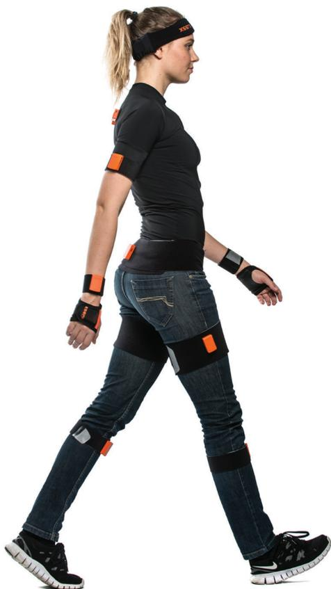
**Figure 19.** A subject instrumented with Xsens wearable inertial sensor technology. (Reprinted with permission from Xsens Technologies B.V., Enschede, The Netherlands. © 2015.)
