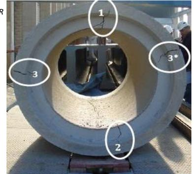
1. The mechanical response of the pipe could be modelled by considering only a quarter of circle (because of the double symmetry existing) and two plastic hinges (one in the crown and other in the haunch) which control the non linear behaviour of the pipe
