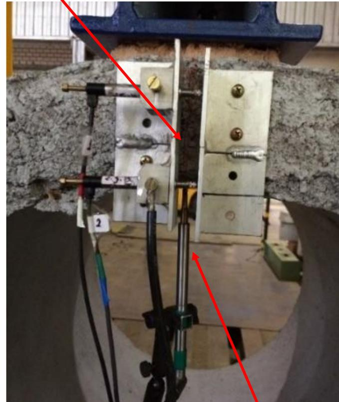
Diametric displacement measurement
