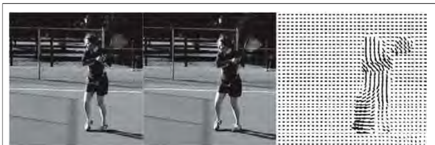
Figure 24.10 Two frames of a video sequence. On the right is the optical flow field corresponding to the displacement from one frame to the other. Note how the movement of the tennis racket and the front leg is captured by the directions of the arrows. (Courtesy of Thomas Brox.)
