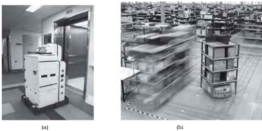
Figure 2517 (a) The Helpmate robot transports food and other medical items in dozens of hospitals worldwide. (b) Kiva robots are part of a material-handling system for moving shelves in fulfillment centers. Image courtesy of Kiva Systems.
