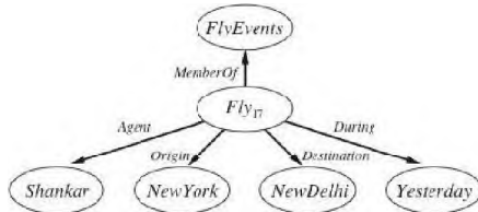
Figure 12.6 A fragment of a semantic network showing the representation of the logical assertion Fly(Shankar, NewYork, NewDelhi, Yesterday) .
