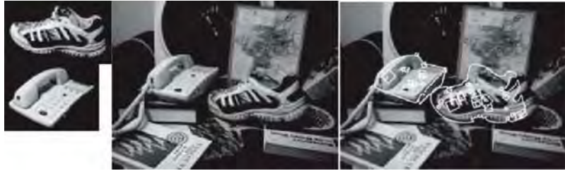
Figure 24.15 Another example of object recognition, this one using the SIFT feature (Scale Invariant Feature Transform), an earlier version of the HOG feature. On the left , images of a shoe and a telephone that serve as object models. In the center, a test image. On the right , the shoe and the telephone have been detected by: finding points in the image whose SIFT feature descriptions match a model; computing an estimate of pose of the model; and verifying that estimate. A strong match is usually verified with rare false positives. Images from Lowe (1999) © IEEE.
