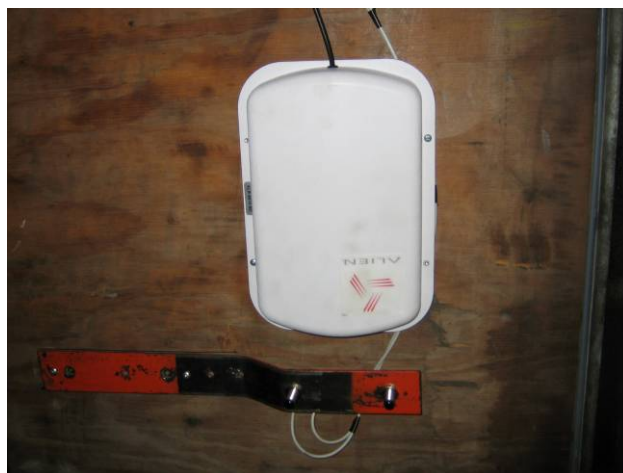
Figure 12: Mounted Antenna and Direction Sensors
