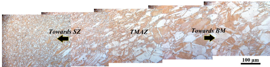
Fig. 3. The combined optical microstructure showing different zones of BM, TMAZ and SZ in advancing side of the joint.
