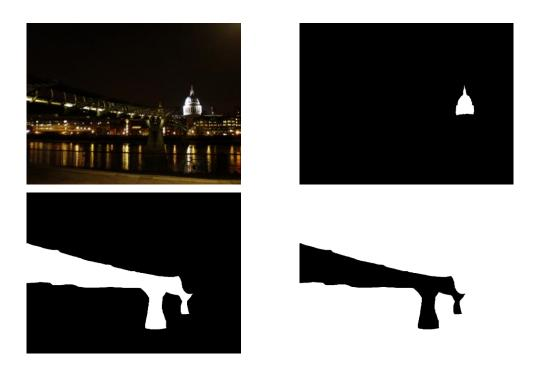
Figure 13. The Millennium Bridge night-time photograph and some of the masks used to calculate the average luminance of target areas in the picture.
