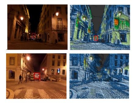
Figure 72. The area of the image (in red) analysed for average luminance in route 1 (top) and 2 (bottom) for node C.
