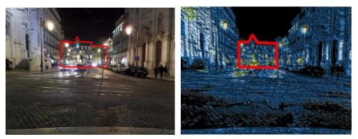
Figure 66. The area of the image (in red) analysed for average luminance on route 1.
