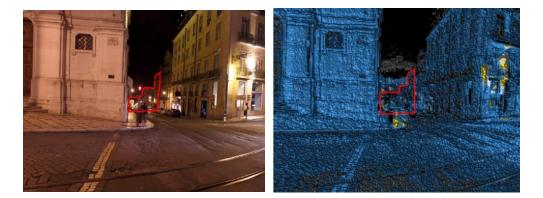
Figure 67. The area of the image (in red) analysed for average luminance on route 2.
