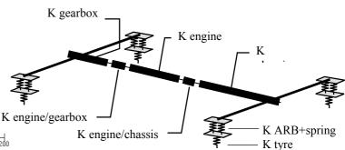
Fig. 4 - Single-seater vehicle model
