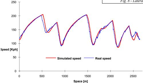
Fig. 7 - Hockenheim ring simulation: speed vs space
