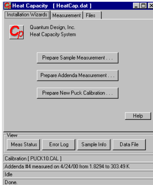
Figure 4-1. Installation Wizards Tab in Heat Capacity Control Center
