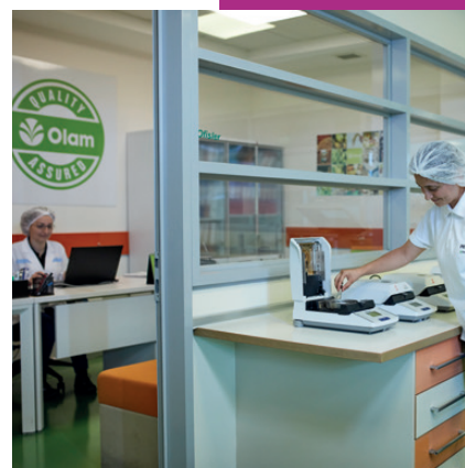
In the Process Control Lab in the Piraziz Integrated Plant in Turkey, the Quality Control staff are analysing the humidity of the processed hazelnuts according to the customer specifications.
