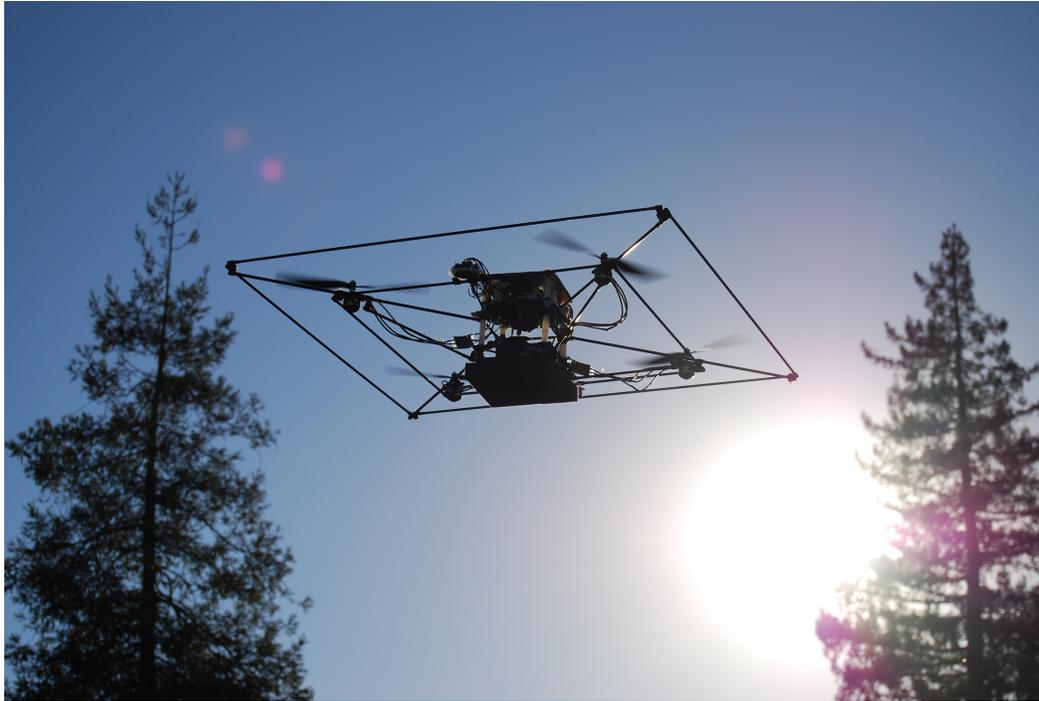
*STARMAC quadrotor aircraft (Tomlin, et al.)*
