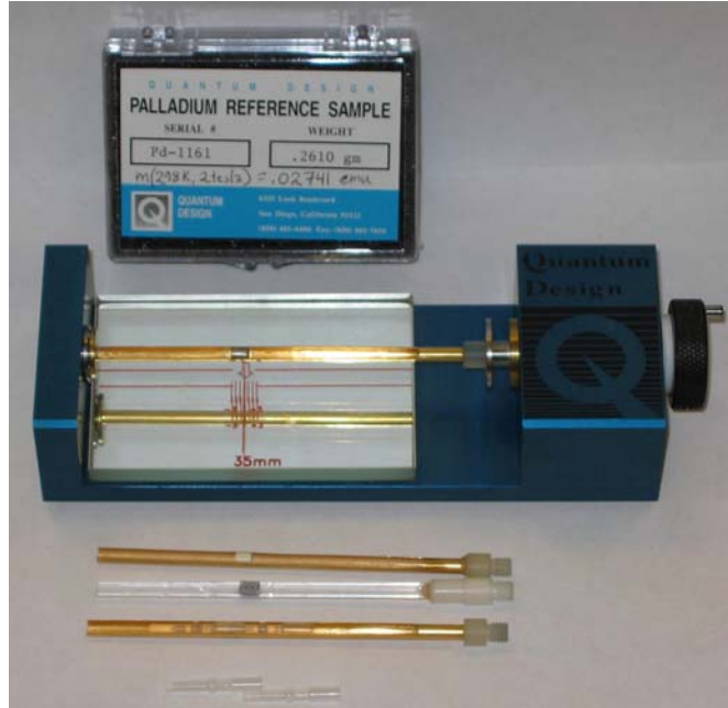
Quantum Design supplied sample holders and PPMS-VSM mounting station.
