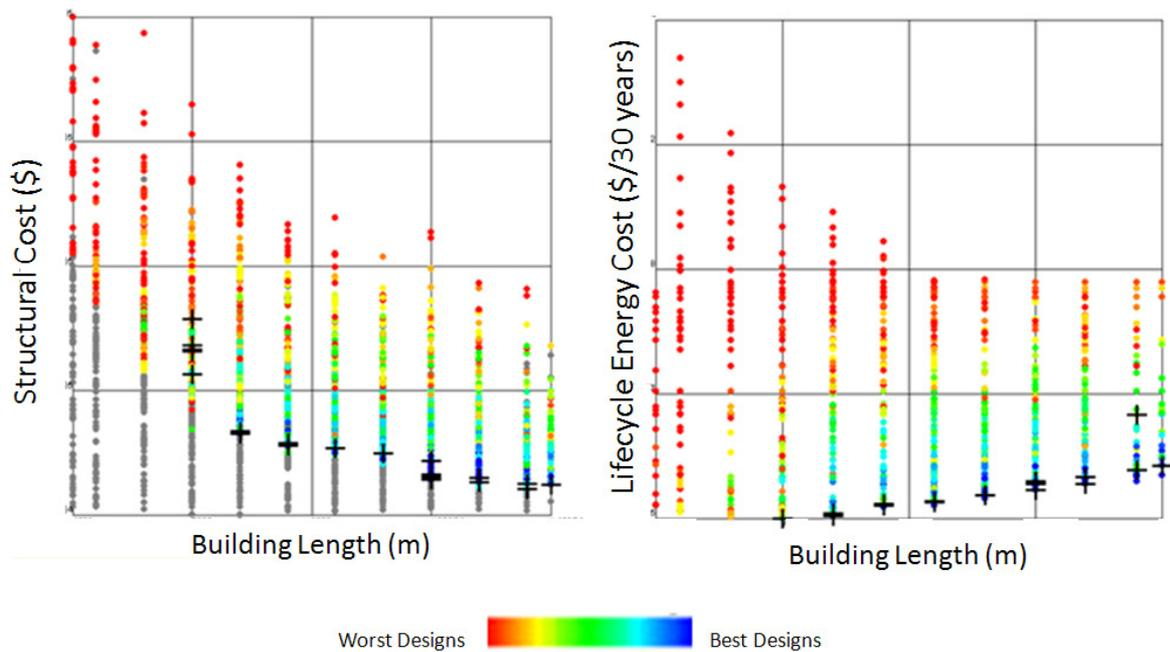
Fig. 11: When structural costs (left) and energy costs (right) are plotted against building length, the Pareto optimal designs show opposite performance trends
