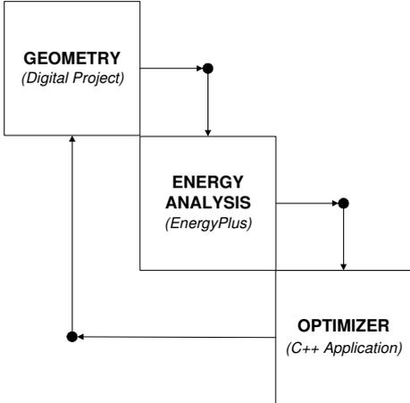
FIG. 6: Energy design, analysis, and optimization process
