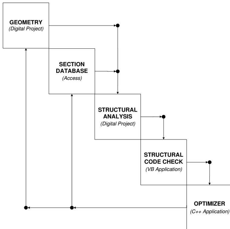
FIG. 3: Structural design, analysis, and optimization process
