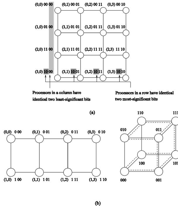
(a) A  $4 \times 4$  mesh illustrating the mapping of mesh nodes to the nodes in a four-dimensional hypercube; and (b) a  $2 \times 4$  mesh embedded into a three-dimensional hypercube.
