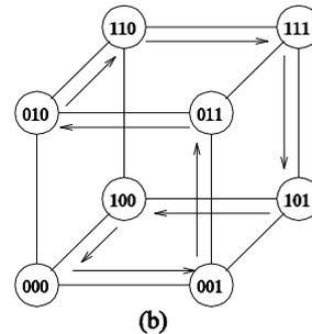
(a) A three-bit reflected Gray code ring; and (b) its embedding into a three-dimensional hypercube.
