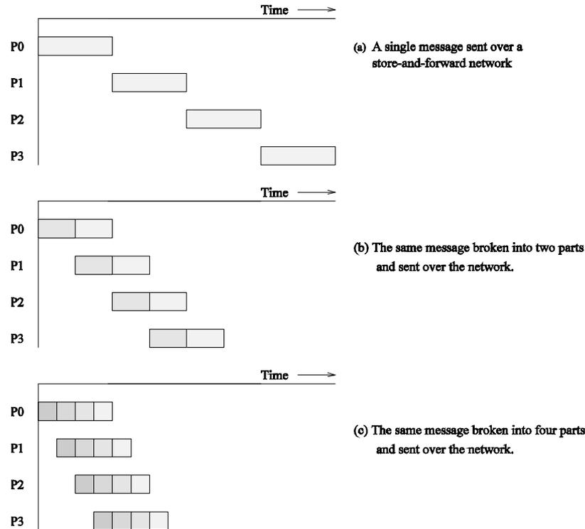
Passing a message from node  $P_0$  to  $P_3$  (a) through a store-and-forward communication network; (b) and (c) extending the concept to cut-through routing. The shaded regions represent the time that the message is in transit. The startup time associated with this message transfer is assumed to be zero.
