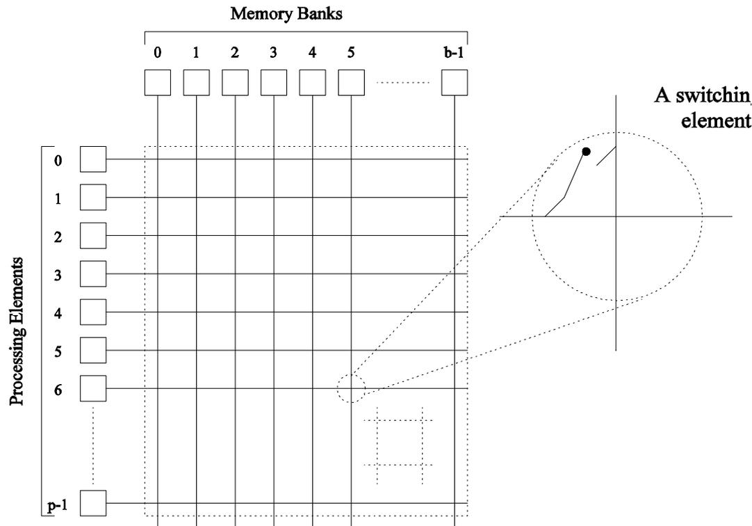
A completely non-blocking crossbar network connecting  $p$  processors to  $b$  memory banks.
