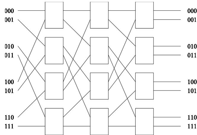
A complete omega network connecting eight inputs and eight outputs.
