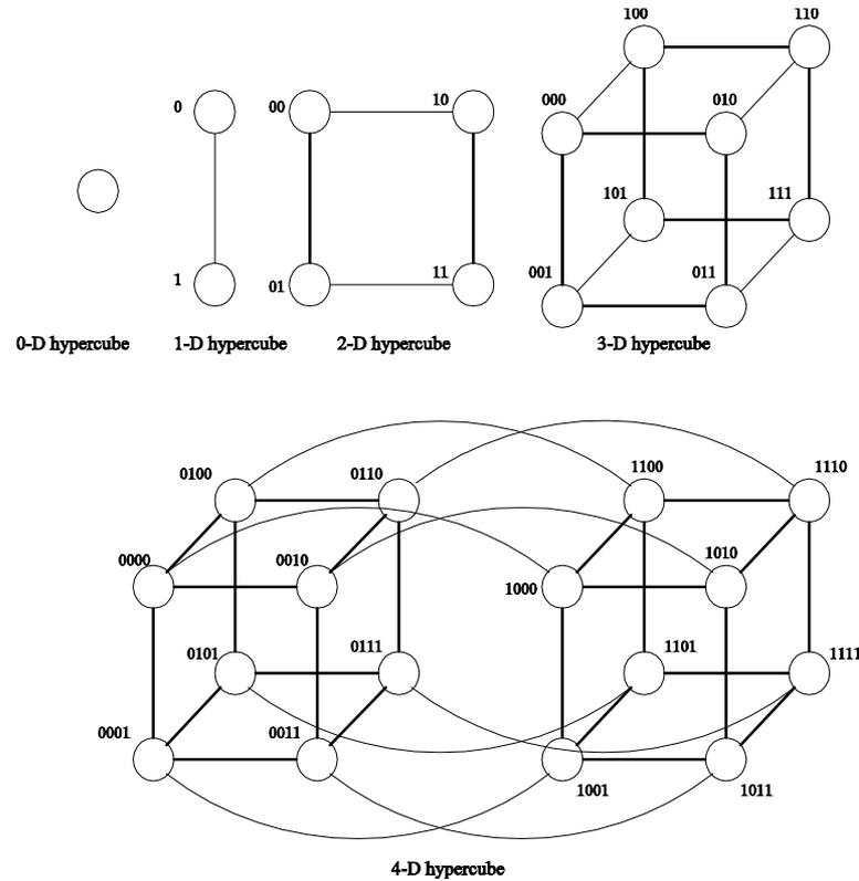
Construction of hypercubes from hypercubes of lower dimension.
