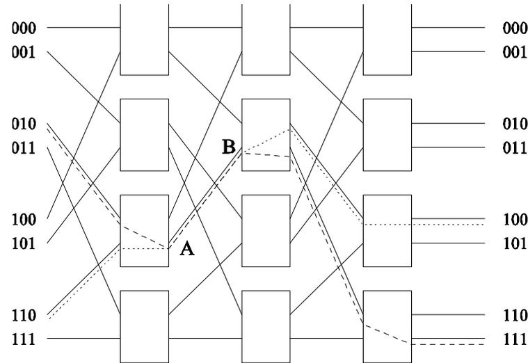
An example of blocking in omega network: one of the messages (010 to 111 or 110 to 100) is blocked at link AB.
