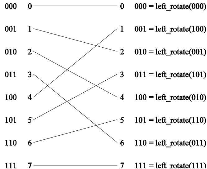
A perfect shuffle interconnection for eight inputs and outputs.
