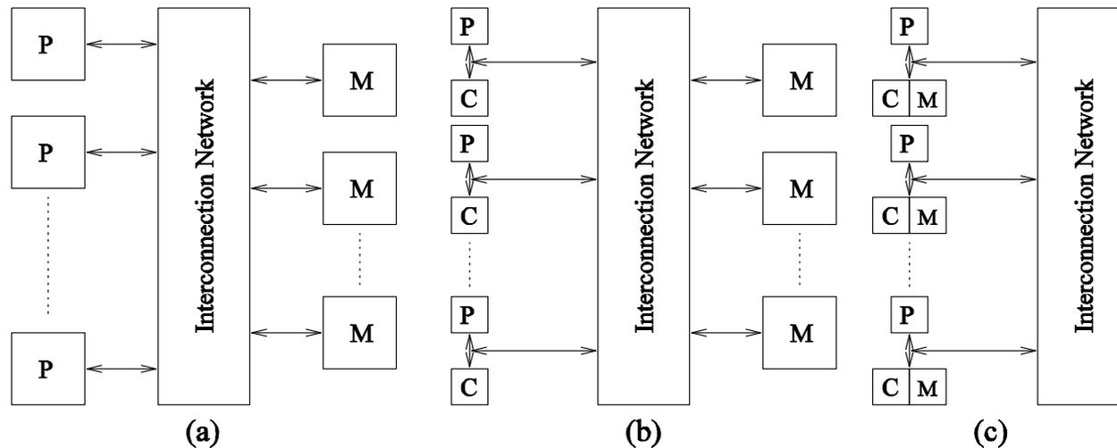
Typical shared-address-space architectures: (a) Uniform-memory access shared-address-space computer; (b) Uniform-memory-access shared-address-space computer with caches and memories; (c) Non-uniform-memory-access shared-address-space computer with local memory only.
