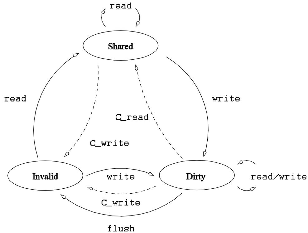
State diagram of a simple three-state coherence protocol.
