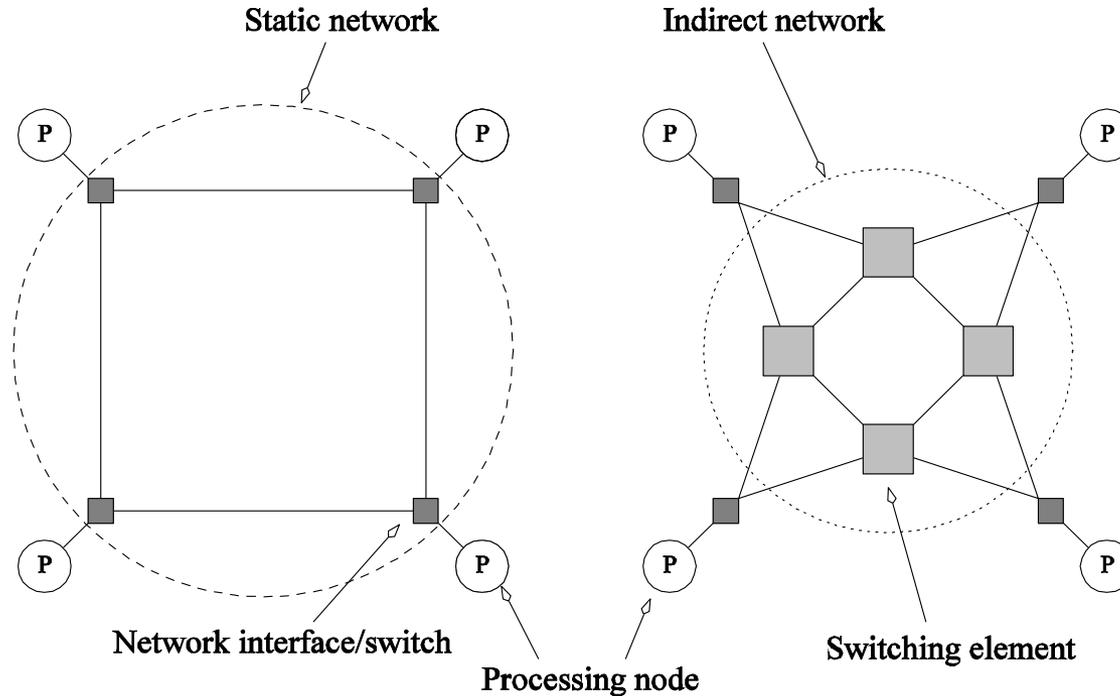
Classification of interconnection networks: (a) a static network; and (b) a dynamic network.
