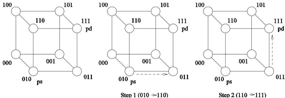
Routing a message from node  $P_s$  (010) to node  $P_d$  (111) in a three-dimensional hypercube using E-cube routing.
