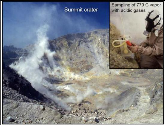
**Sampling of 770 C vapor with acidic gases**
