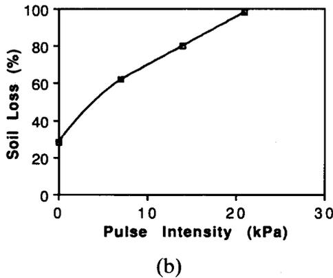
Fig. 5. (a) Dynamic filtration response of lightweight nonwoven needle punched geotextile to various pulse intensities for Le Bow soil with size fraction less than no. 100 sieve (150  $\mu$ m). (b) Loss of soil caused by increase in pulse intensity for lightweight nonwoven needle punched geotextile data from (a).
