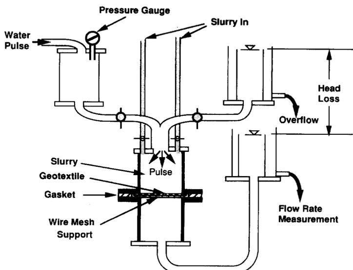
Fig. 1. Schematic diagram of dynamic filtration test set-up.
