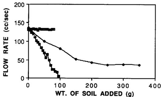
**Fig. 2.** Dynamic filtration test results on lightweight nonwoven needle punched geotextile. □, Fly ash; ◆, well graded sand; ■, Le Bow soil with size fraction less than no. 100 sieve (150  $\mu$ m).
