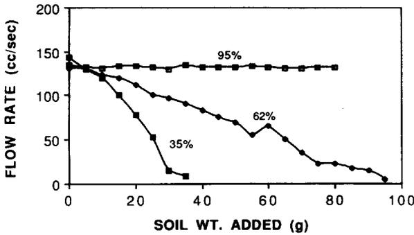
Fig. 3. Dynamic filtration response of lightweight nonwoven needle punched geotextile to various soil sizes.  $\square$ ,  $<$  no. 200 sieve ( $75\ \mu\text{m}$ );  $\blacklozenge$ ,  $<$  no. 100 sieve ( $150\ \mu\text{m}$ );  $\blacksquare$ ,  $<$  no. 80 sieve ( $180\ \mu\text{m}$ ).
