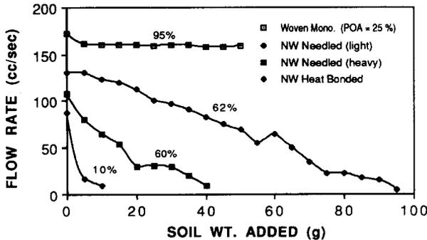
Fig. 4. Dynamic filtration response of various geotextiles to Le Bow soil with size fraction less than no. 100 sieve ( $150\ \mu\text{m}$ ).
