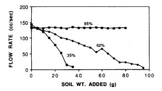
**Fig. 3.** Dynamic filtration response of lightweight nonwoven needle punched geotextile to various soil sizes.  $\Box$ , < no. 200 sieve (75  $\mu$ m);  $\blacklozenge$  < no. 100 sieve (150  $\mu$ m);  $\Box$ , < no. 80 sieve (180  $\mu$ m).
