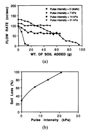
Fig. 5. (a) Dynamic filtration response of lightweight nonwoven needle punched geotextile to various pulse intensities for Le Bow soil with size fraction less than no. 100 sieve (150  $\mu$ m). (b) Loss of soil caused by increase in pulse intensity for lightweight nonwoven needle punched geotextile data from (a).
