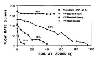
Fig. 4. Dynamic filtration response of various geotextiles to Le Bow soil with size fraction less than no. 100 sieve  $(150 \,\mu m)$ .
