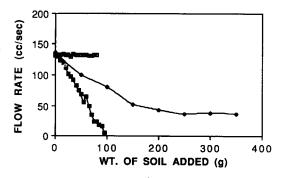
Fig. 2. Dynamic filtration test results on lightweight nonwoven needle punched geotextile. □, Fly ash; ♦, well graded sand; ■, Le Bow soil with size fraction less than no. 100 sieve (150 µm).
