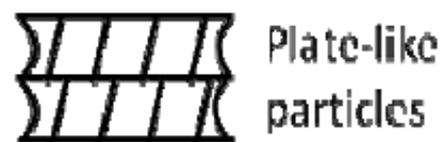
Slits with planar walls, adsorption branch similar to that for nonporous materials; desorption from cylindrical pores.
