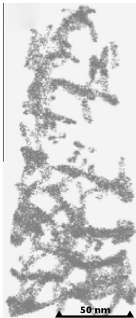
**Fig. 5.10.** Segregation of Mn to a dislocation network in the ODS ferritic steel ODS Eurofer 97 irradiated by  $\text{Fe}^{2+}$  ions to a dose of 2 dpa at 400 °C; from Williams et al. [103].
