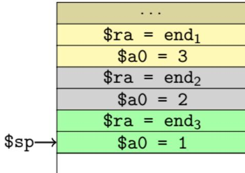
The diagram illustrates the execution stack with three frames. The stack grows downwards. The bottom frame is green and contains the value \$a0 = 1. The middle frame is grey and contains the value \$a0 = 2. The top frame is yellow and contains the value \$a0 = 3. Above the stack, the register \$ra is shown with its values for each frame: end<sub>3</sub>, end<sub>2</sub>, and end<sub>1</sub>. An arrow points from the label \$sp to the bottom of the stack.
